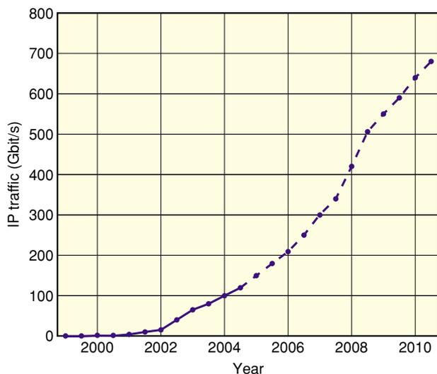
Fig. 2. Trend and estimate of IP traffic on backbone network.
