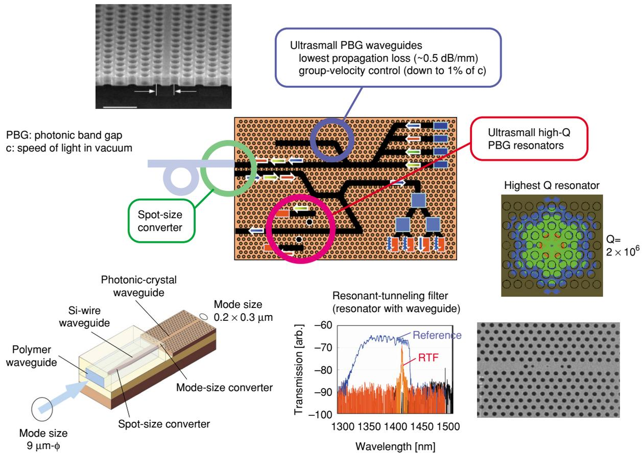
Fig. 3. Schematic of integrated optical circuit using photonic crystal.
