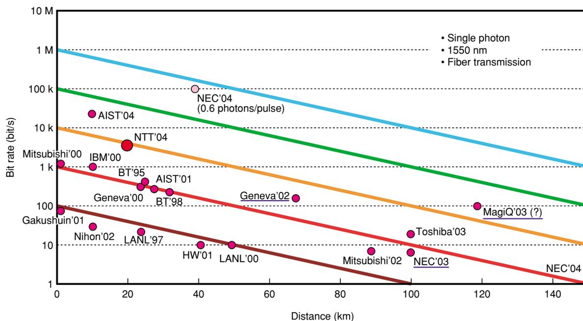
Fig. 6. Comparison of key generation rates and transmission distances of quantum cryptography methods.
