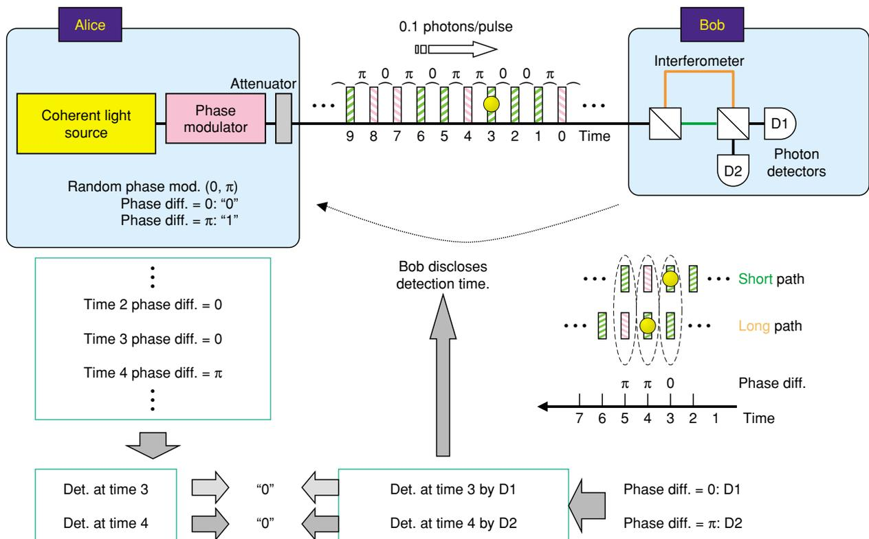
Fig. 5. Setup and protocol of differential phase shift quantum key distribution (DPS-QKD).
