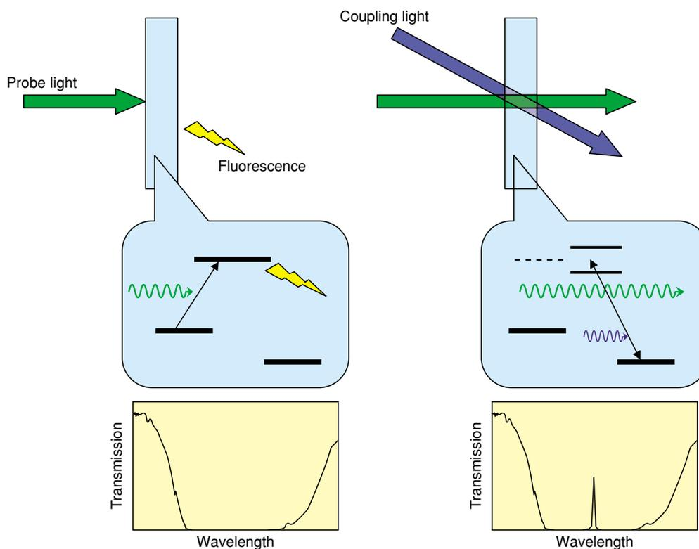
Fig. 4. Schematic of electromagnetically induced transparency.
