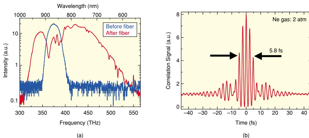
Fig. 6. A few-cycle laser pulse under gas pressure of 2 atm in a hollow fiber. (a) Laser spectra before and after the hollow fiber. (b) Autocorrelation signal.
