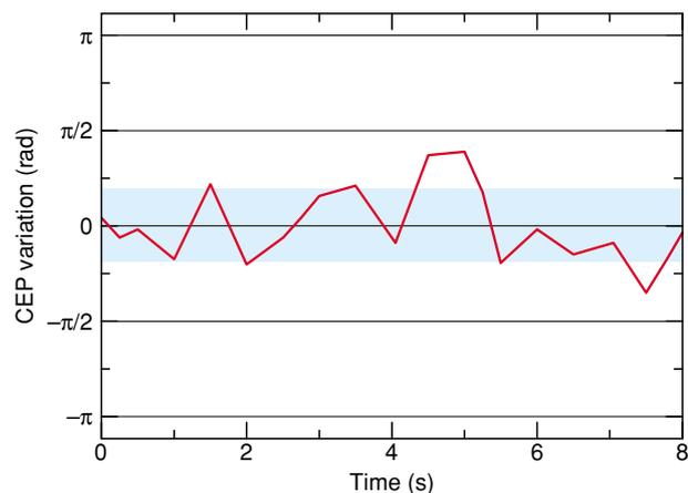
Fig. 8. CEP variations after the hollow fiber using a multi-pass amplifier with the CEP-slip-controlled oscillator. The gas pressure in the hollow fiber was 2 atm. The width of the blue zone shows the standard deviation of the CEP drifts.
