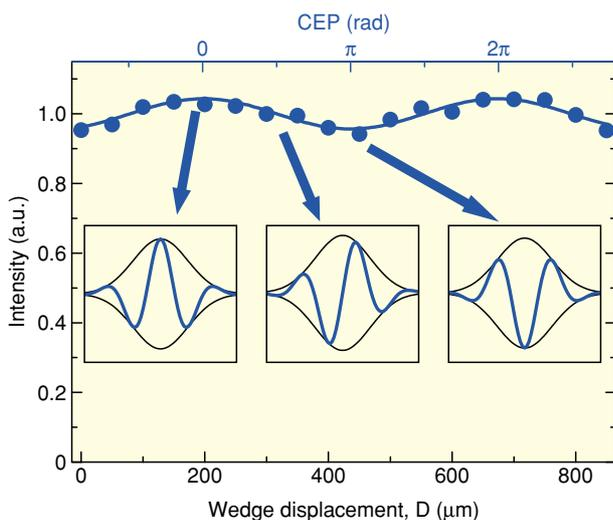
Fig. 9. Interference intensity as a function of the change in path length through the fused silica glass wedges (Fig. 5).
