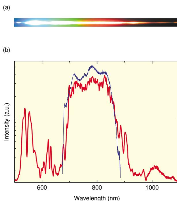
Fig. 3. Propagation in the photonic-crystal fiber broadens the spectrum to more than one octave by self-phase modulation. (a) Photograph and (b) spectrograph before (blue line) and after (red line) the photonic-crystal fiber.
