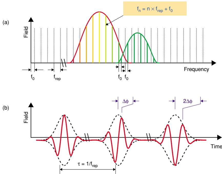
Fig. 2. Time-frequency correspondence and relationship between  $\Delta\phi$  and  $f_0$ . (a) In the frequency domain, the elements of the frequency comb of a mode-locked pulse train have a spacing of  $f_{rep}$ . (b) In the time domain, the three pulses are part of an infinite train with a constant  $\Delta\phi$  when the pulse-to-pulse CEP slips are controlled.
