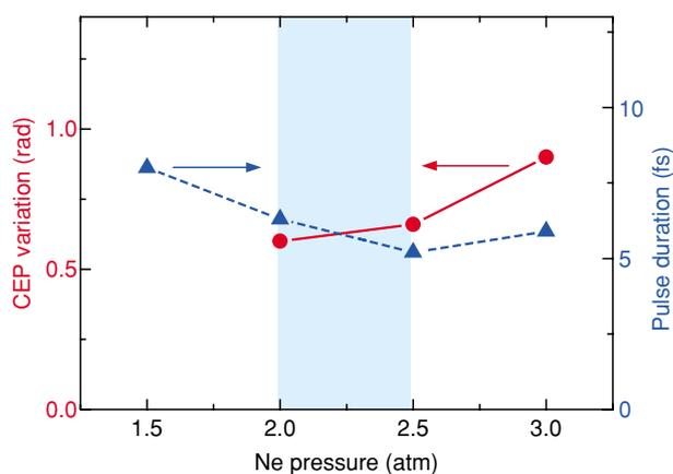
Fig. 7. Relationship between the laser pulse width and the CEP variations in the experiment.
