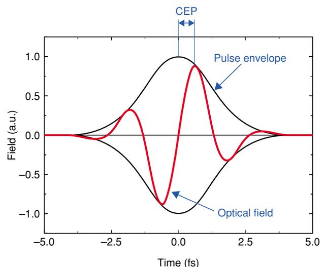
Fig. 1. Ultrashort laser pulse: The pulse intensity envelope is shown by the black line and the oscillating electric field by the red line.
