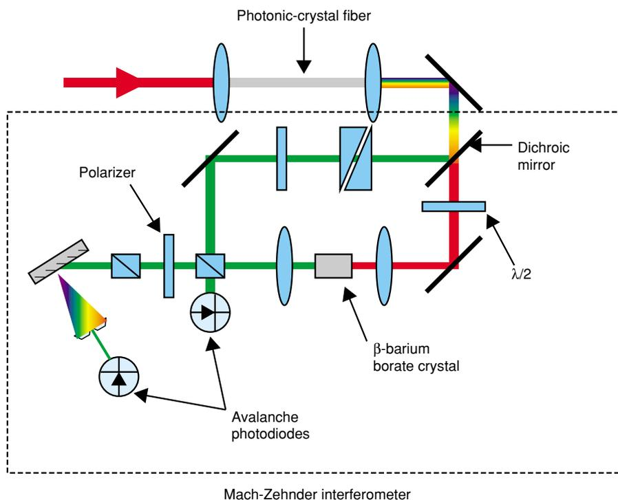
Fig. 4. The  $f$ -to- $2f$  interferometer used in the measurement of  $f_o$ .
