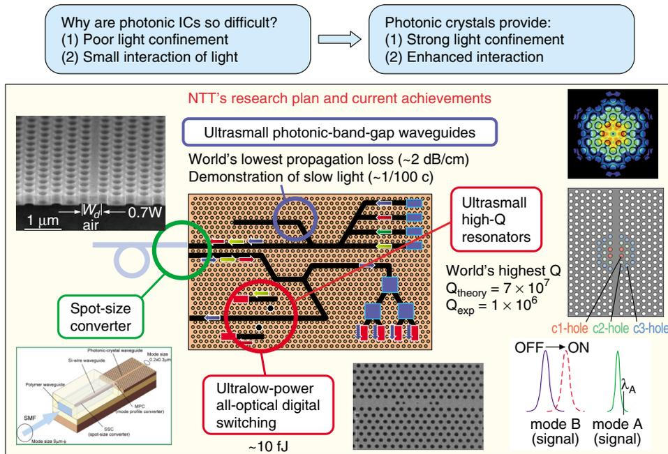
Fig. 2. Photonic integrated circuits on photonic-crystal platform.
