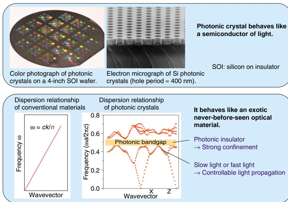
Fig. 1. Photonic crystals as new artificial optical materials.
