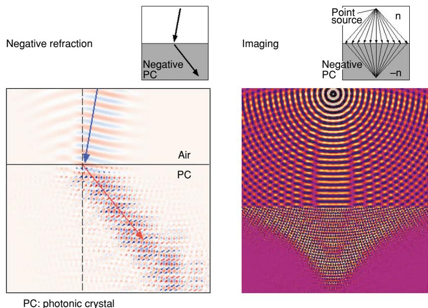
Fig. 3. Negative refraction in photonic crystals.
