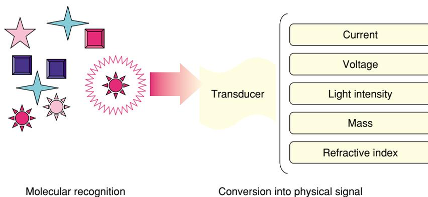
Fig. 2. Elements of chemical sensor.
