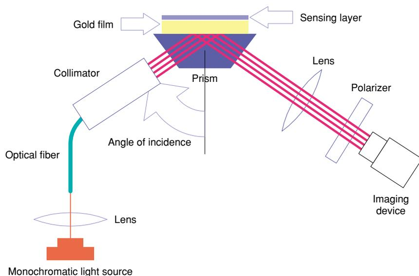
Fig. 8. Optical configuration for imaging SPR.
