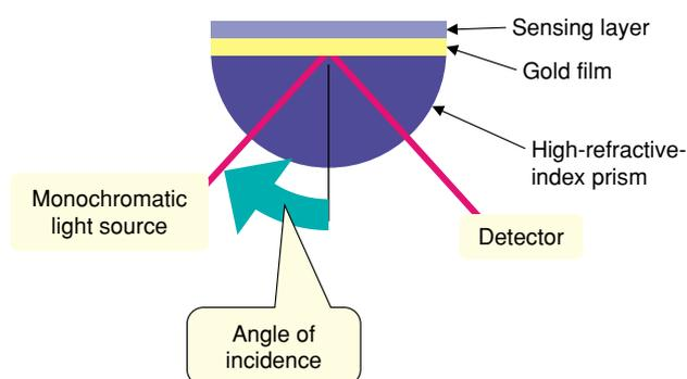
Fig. 4. Measurement of refractive index by SPR.
