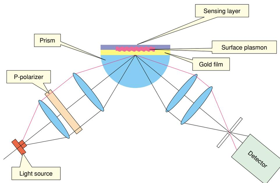
Fig. 7. Optical setup for SPR.
