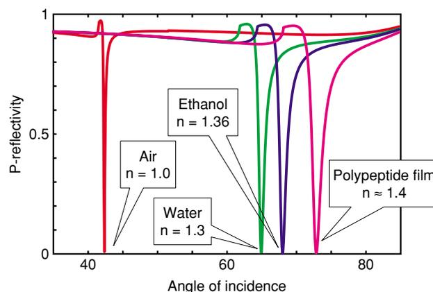
Fig. 5. SPR curves for different molecules ( $n$  = refractive index).
