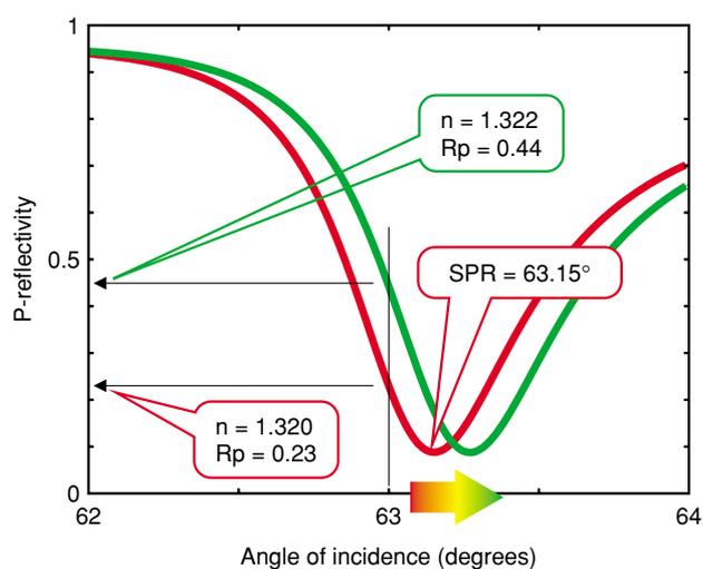
Fig. 9. Refractive index mapping.
