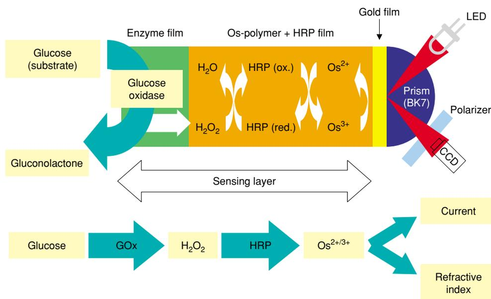
Fig. 10. Structure of SPR enzyme-based sensor.
