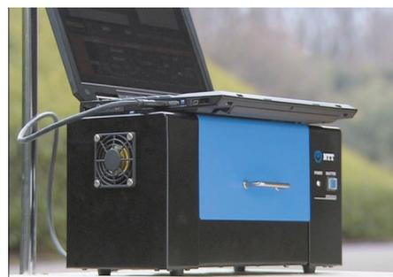
Fig. 2. Portable VOC sensor developed by NTT.
