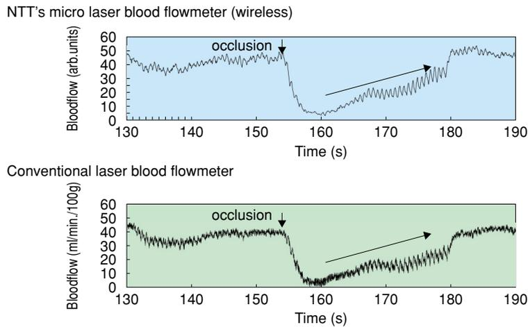
Fig. 7. Bloodflow data obtained with NTT's micro laser blood flowmeter and with a conventional one.
