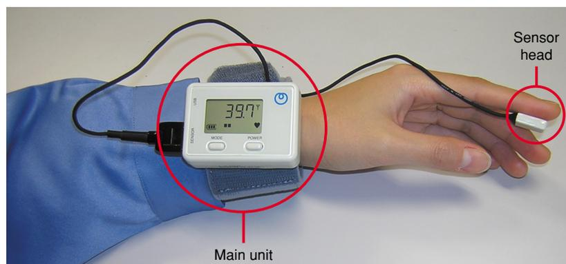
Fig. 6. Micro laser blood flowmeter.
