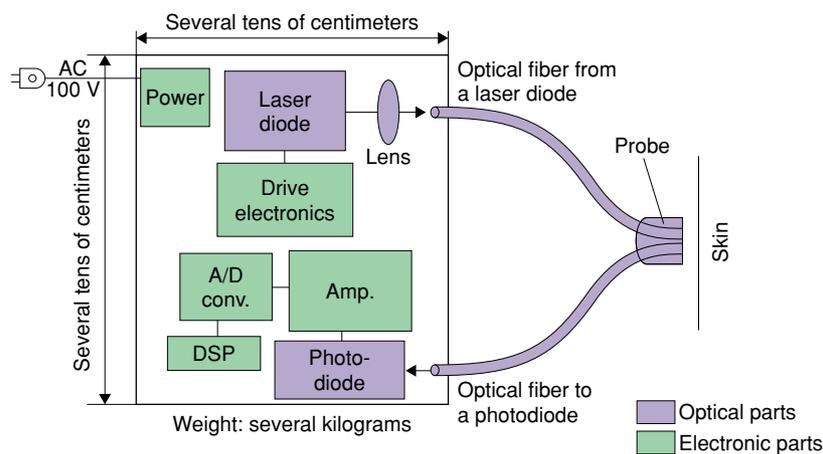
Fig. 3. Structure of a conventional laser blood flowmeter.
