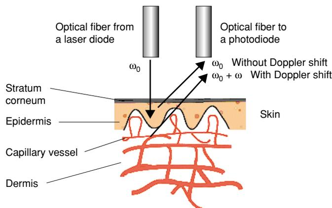
Fig. 1. Principle of laser blood flow measurement.
