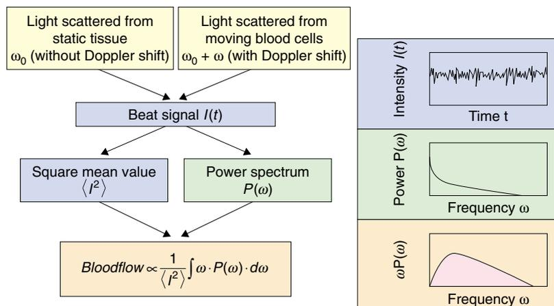
Fig. 2. Principle of bloodflow calculation.
