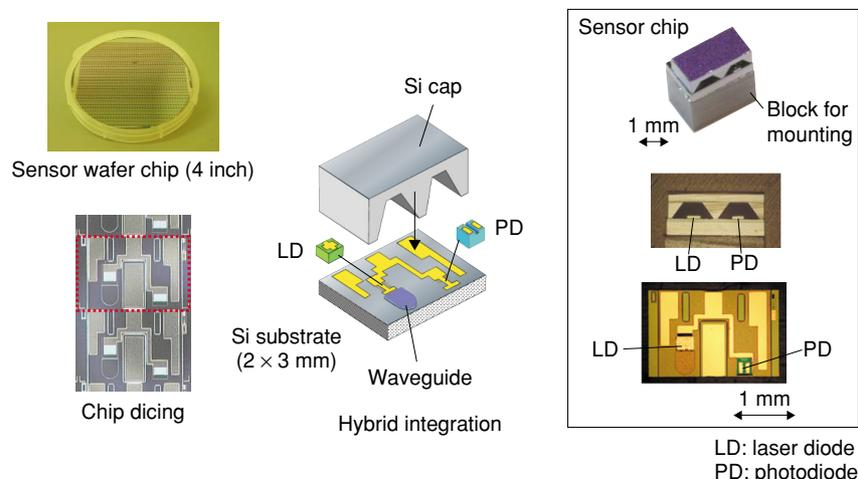
Fig. 4. Fabrication process and sensor structure.
