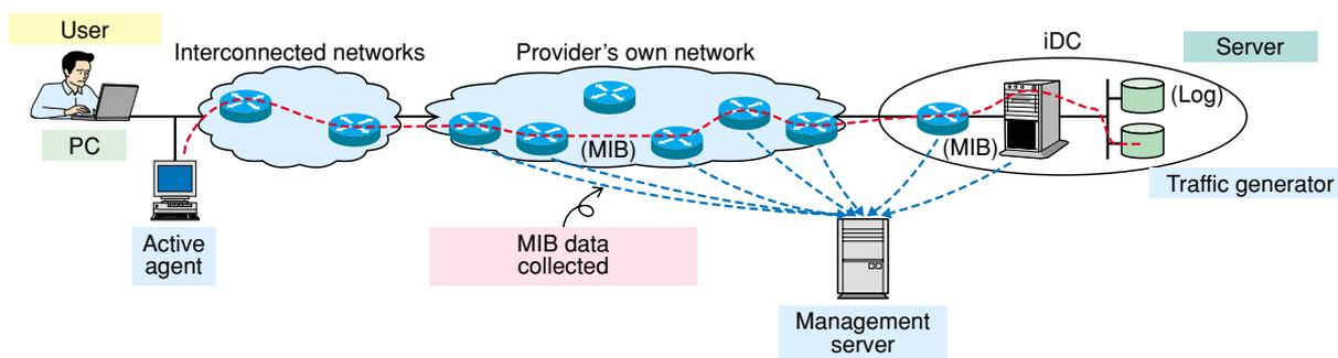
Fig. 5. Scheme for pinpointing bottlenecks.
