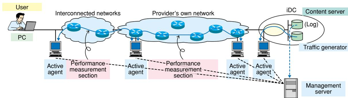
Fig. 4. Scheme for localizing degraded sections.
