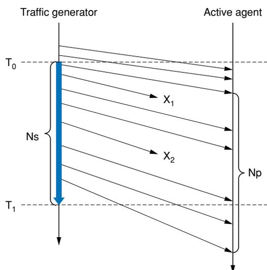
Fig. 2. Definition of packet loss ratio.
