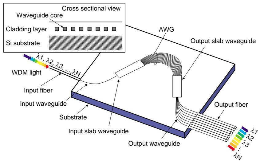
Fig. 1. AWG-type wavelength multiplexer/demultiplexer using PLC. Input light is demultiplexed into different outputs thanks to the prism-like dispersion function of the AWG.
