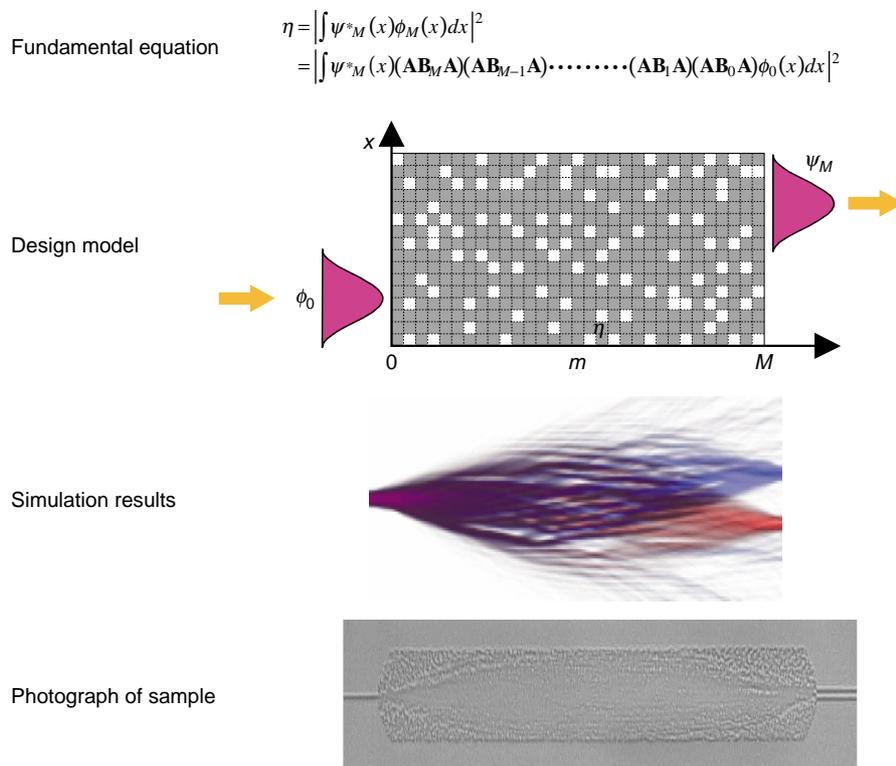
Fig. 2. Generation of waveguide pattern by wavefront matching method. A waveguide pattern is automatically designed by inverse-calculation for maximum  $\eta$ . The pattern shown in the picture can separate 1.3- and 1.5- $\mu\text{m}$  lights.
