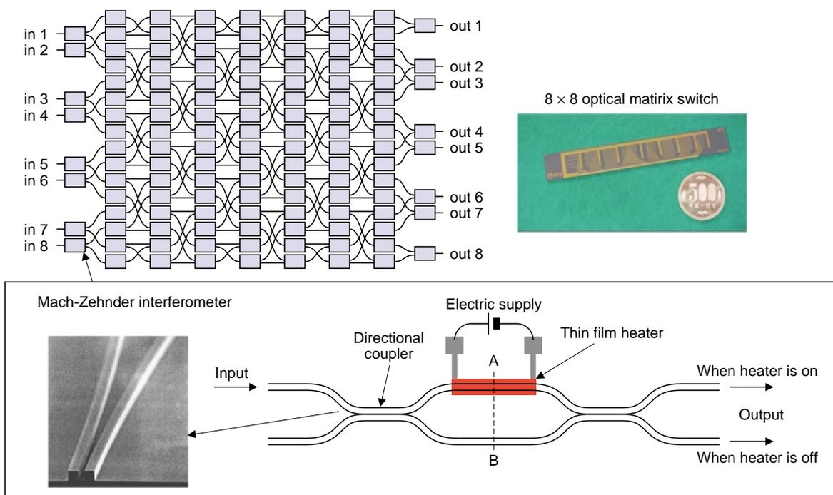
Fig. 3. Structure of a Mach-Zehnder-interferometer optical switch ( $8 \times 8$ ). The device divides input light along two optical waveguides and switches the output port according to the phase difference between the two signals after merging. A phase difference is generated by changing the temperature of a waveguide using a heater (on/off operation). Integrating a large number of these switches (as shown by the matrix switch in the upper left) leads to large-scale switching.
