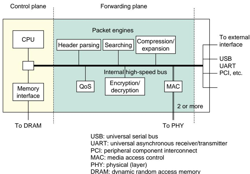
Fig. 4. General configuration of the network processor.
