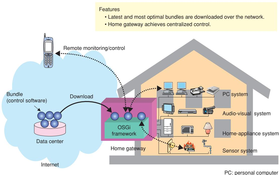
Fig. 2. OSGi control model (using a home gateway as an example).
