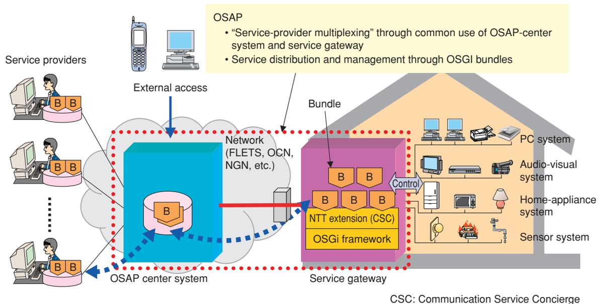
Fig. 3. Outline of OSGi Service Aggregation Platform (OSAP) (using home services as an example).
