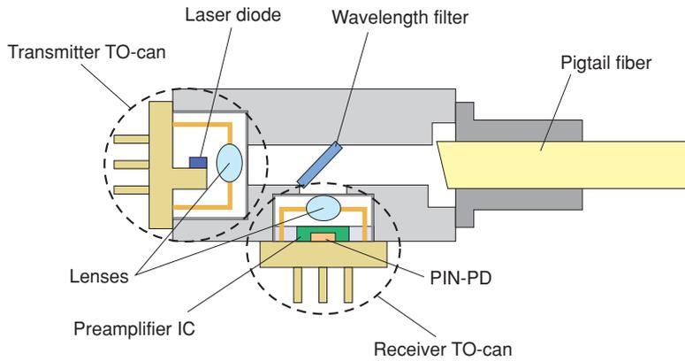
Fig. 2. Bi-directional optical transceiver.
