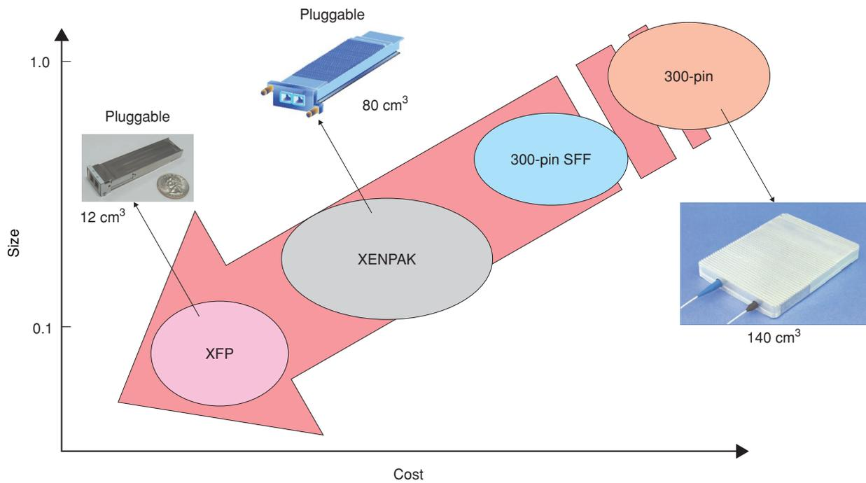
Fig. 1. MSAs of 10-Gbit/s optical transceivers.
