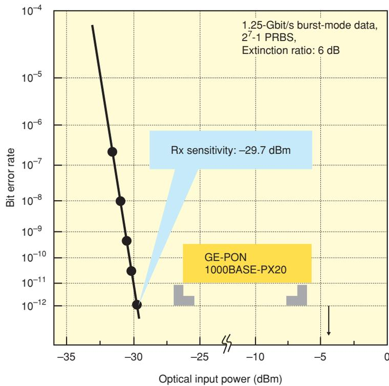
Fig. 6. Bit error rate of the OLT transceiver.
