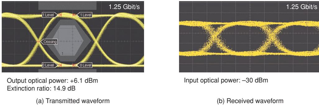
Fig. 5. Waveforms of the OLT transceiver.
