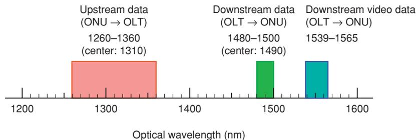
Fig. 3. Optical wavelength allocation in a PON system.
