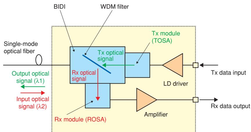
Fig. 1. Configuration of a transceiver.
