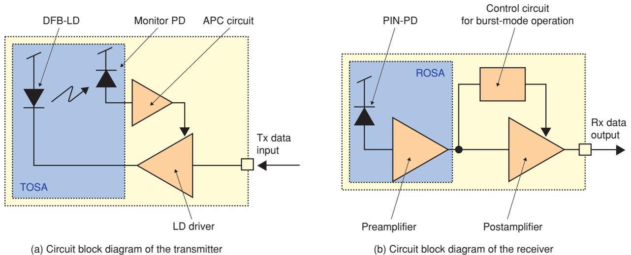
Fig. 2. Block configuration of the transceiver.
