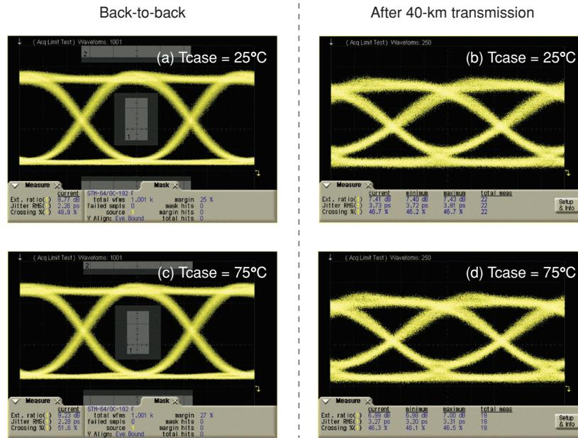
Fig. 3. Eye diagrams for 10.7 Gbit/s NRZ-PRBS  $2^{31}-1$ .
