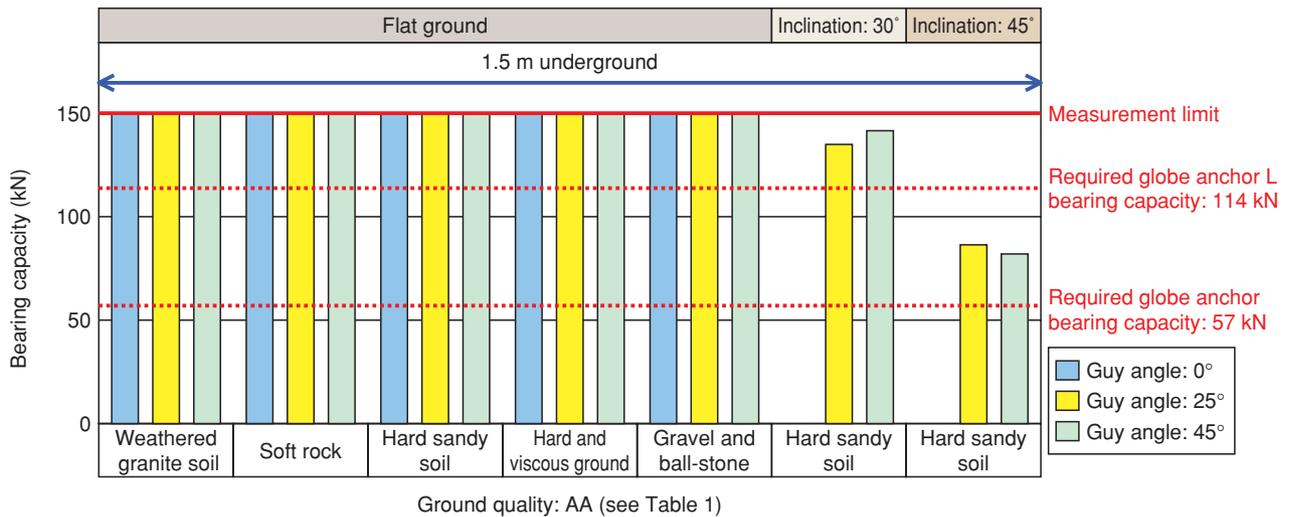
Fig. 6. Bearing capacity in a hard foundation.
