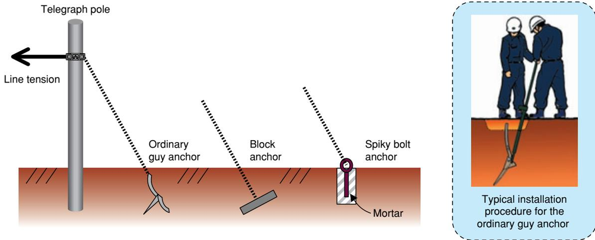
Fig. 1. Existing types of guy anchors.
