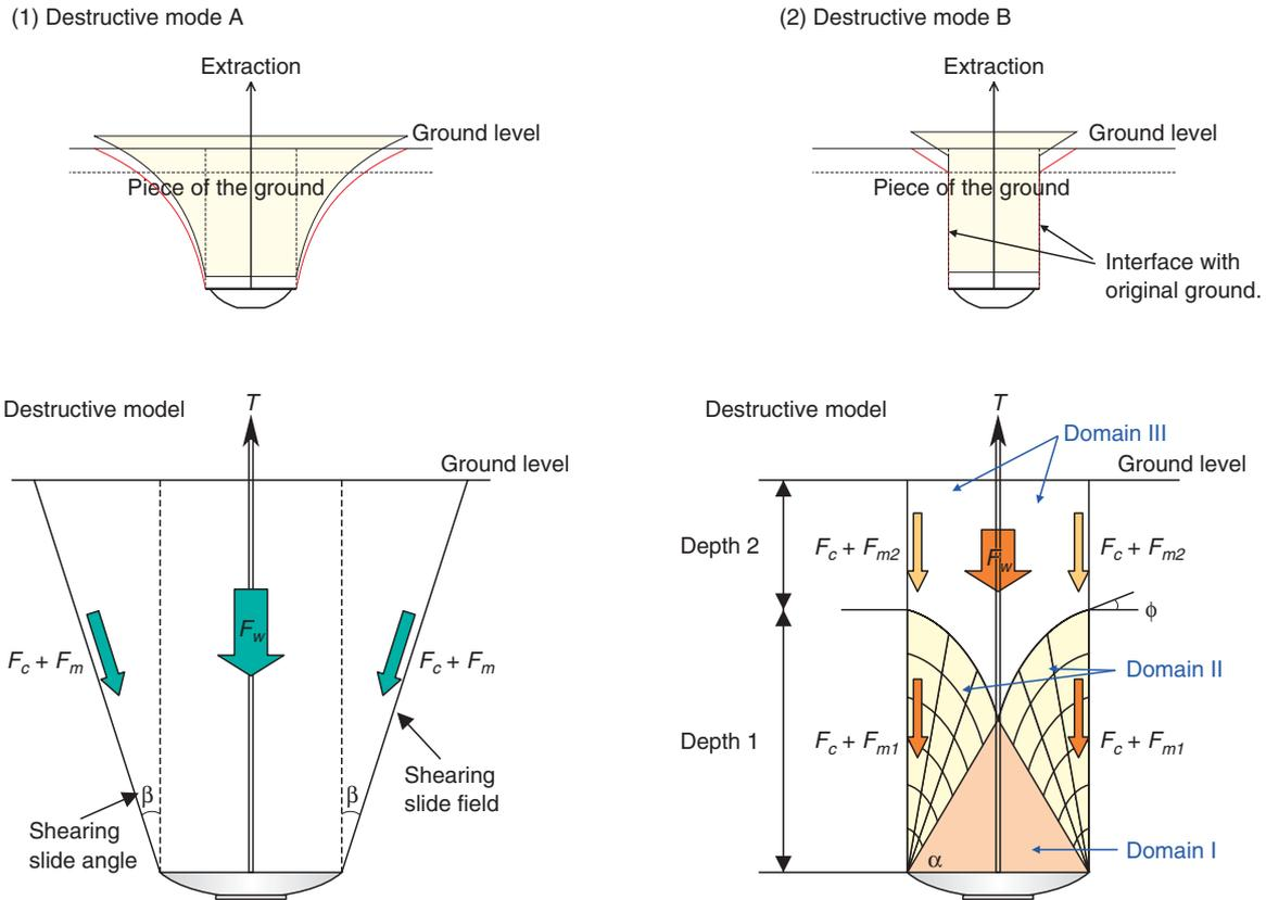
Fig. 4. Modes of destruction of ground holding the globe anchor.
