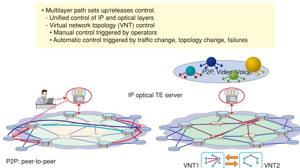
Fig. 2. IP optical multilayer traffic engineering.
