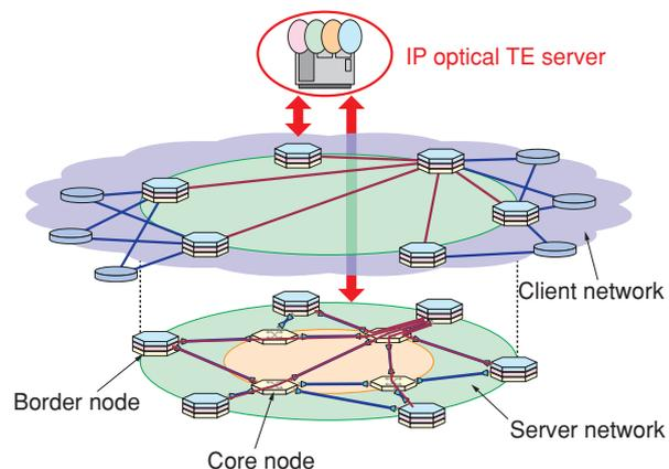
Fig. 1. IP optical multilayer network (MLN).
