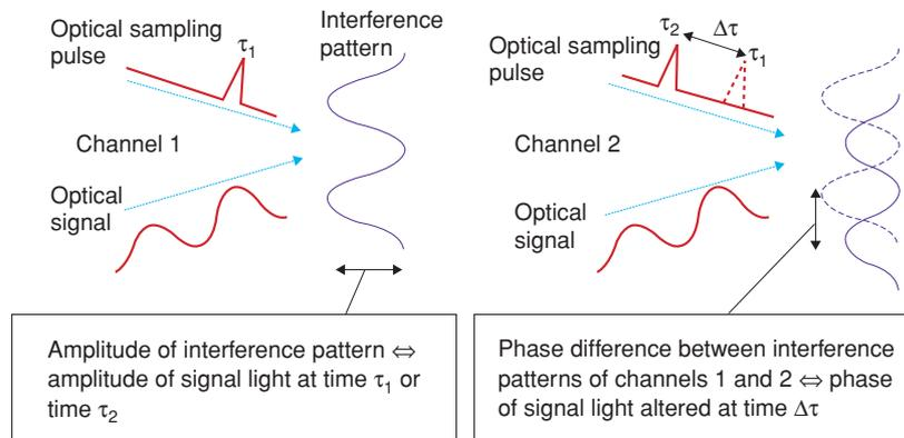
Fig. 1. Principle of linear optical sampling.
