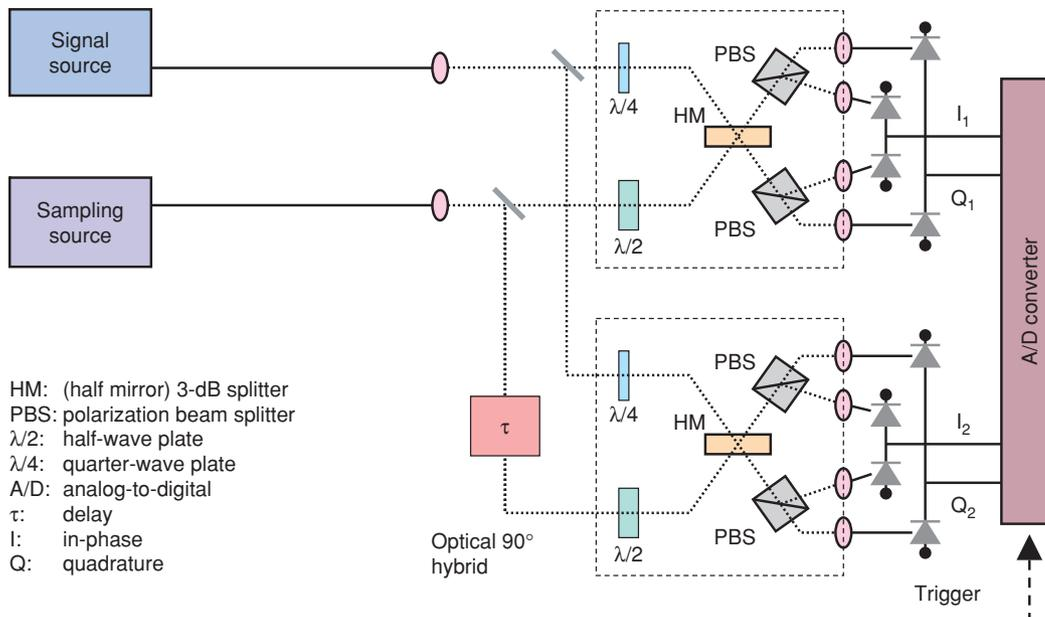
Fig. 2. Equipment configuration.
