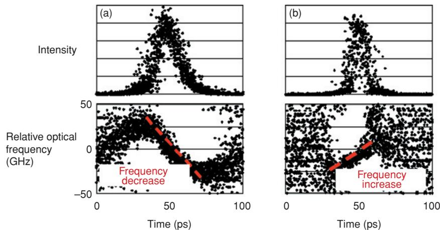
Fig. 3. Experimental results for linear optical sampling.
