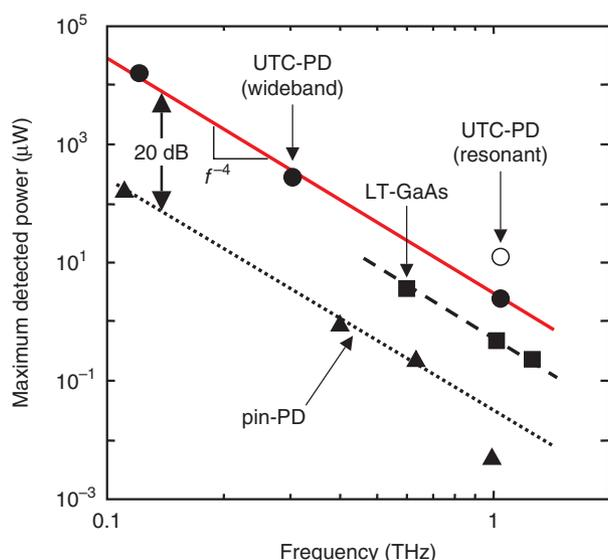
Fig. 7. Comparison of CW output power (average power).
