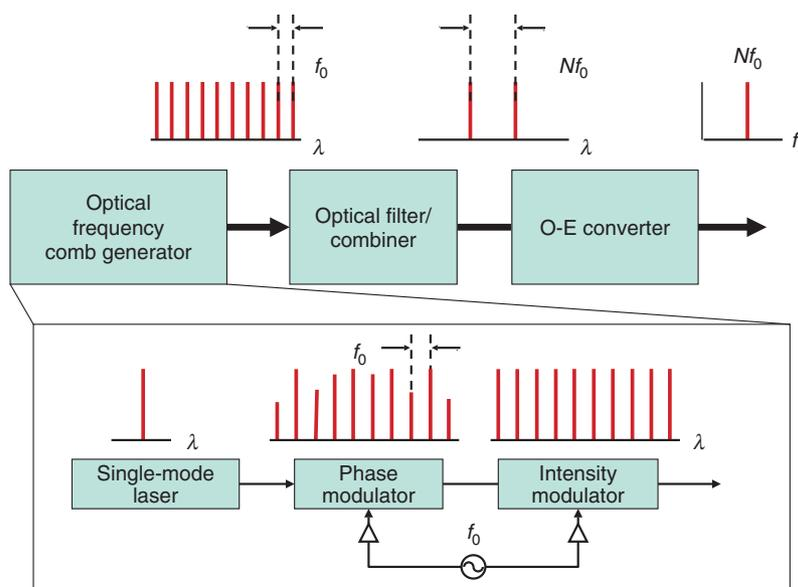
Fig. 3. Block diagram of the MMW/THz-wave generator based on optical heterodyning using optical frequency comb generator.
