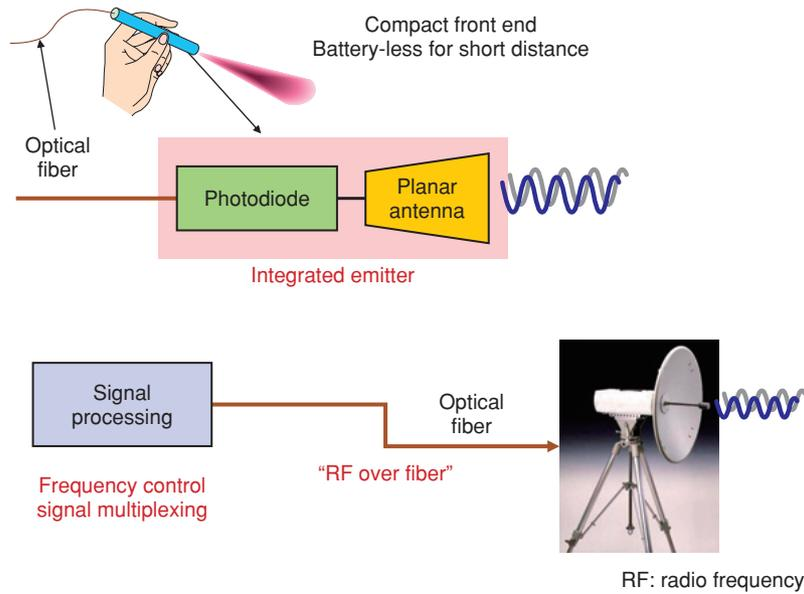
Fig. 1. Conceptual illustration of photonic MMW/THz-wave generators.
