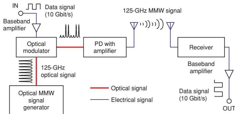
Fig. 10. 120-GHz-band wireless link system using photonic MMW transmitter.
