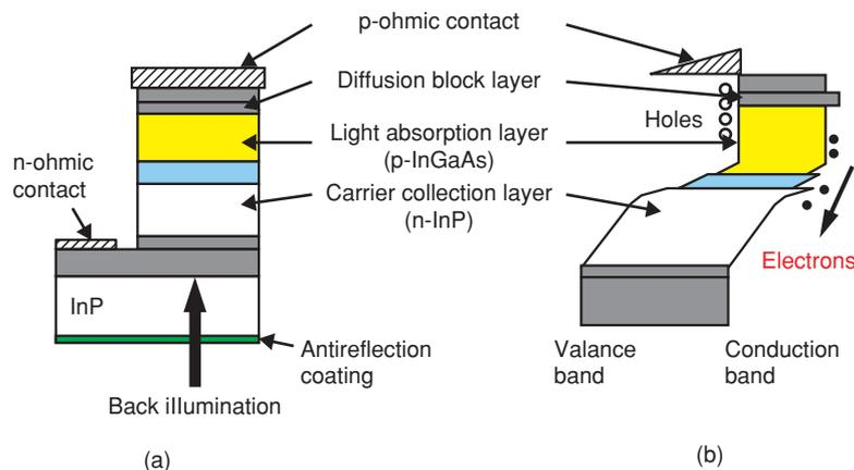
Fig. 6. Structure of UTC-PD. (a) Layer structure and (b) band diagram.
