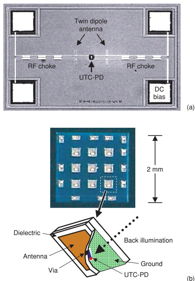
Fig. 8. (a) THz UTC-PD with twin-dipole antenna and (b) microstrip antenna array integrated with UTC-PD.
