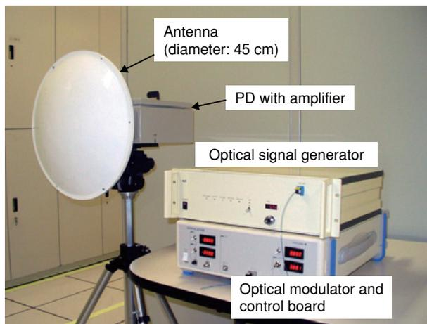
Fig. 11. MMW transmitter for long-distance wireless link.
