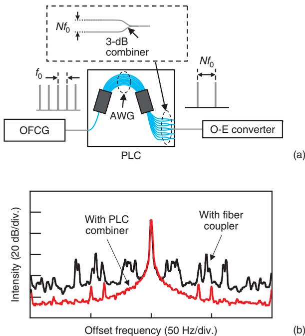
Fig. 5. (a) Role of PLC in photonic MMW generator. (b) RF spectra.
