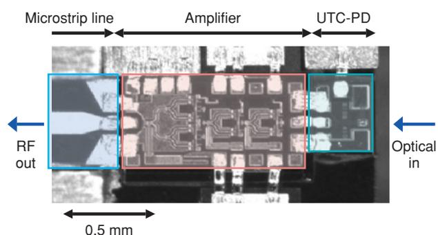
Fig. 9. UTC-PD integrated with power amplifier.
