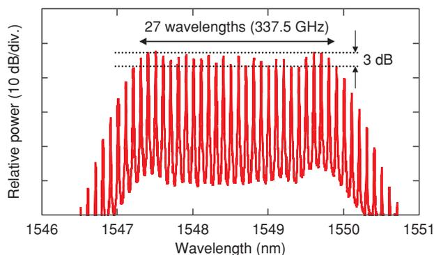
Fig. 4. Optical spectrum of the OFCG. The driving frequency for modulators was 12.5 GHz.
