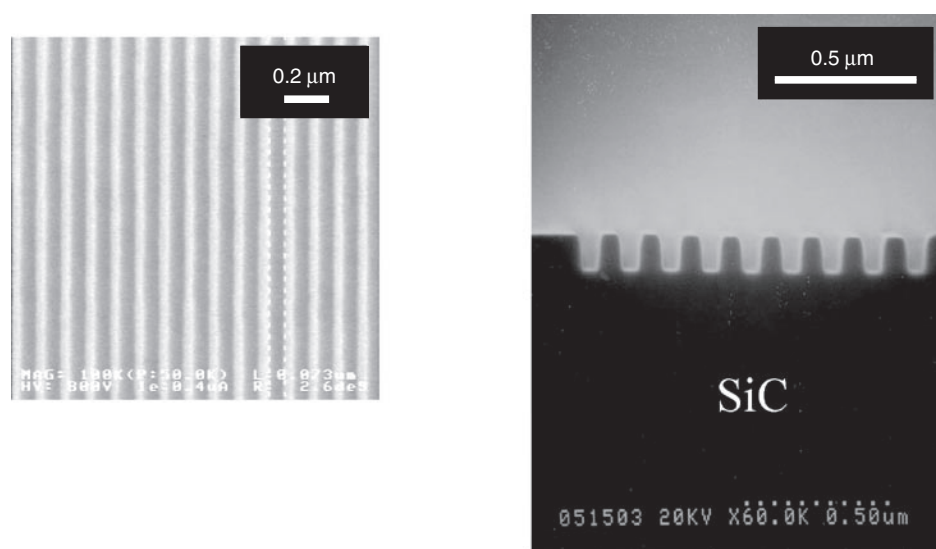
Fig. 7. SEM images of mold patterns: top (left) and cross-sectional (right) views. The top and cross-sectional views are 60- and 80-nm L/S patterns, respectively.
