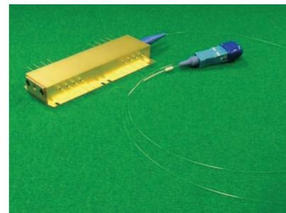
Fig. 6. Photograph of wavelength conversion module.
