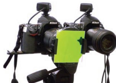
Fig. 10. Filter is mounted in front of the lens of one camera.
