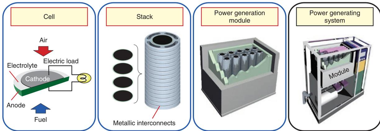
Fig. 1. Configuration of SOFC power generation system.
