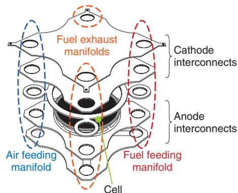
Fig. 2. Configuration of SOFC power generation unit.
