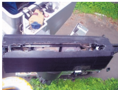
Fig. 4. Damage to an FFA closure (by a squirrel).
