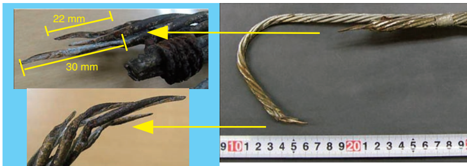
Fig. 1. Fractured aluminium corrosion-resistant wire grip.
