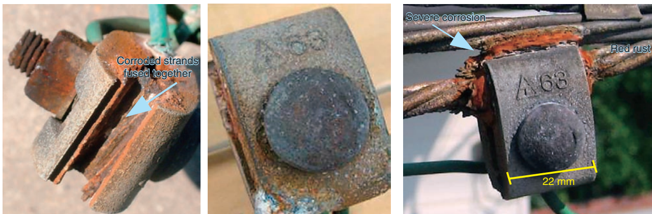
Fig. 2. Ground clamp (on the side opposite the fractured wire grip).
