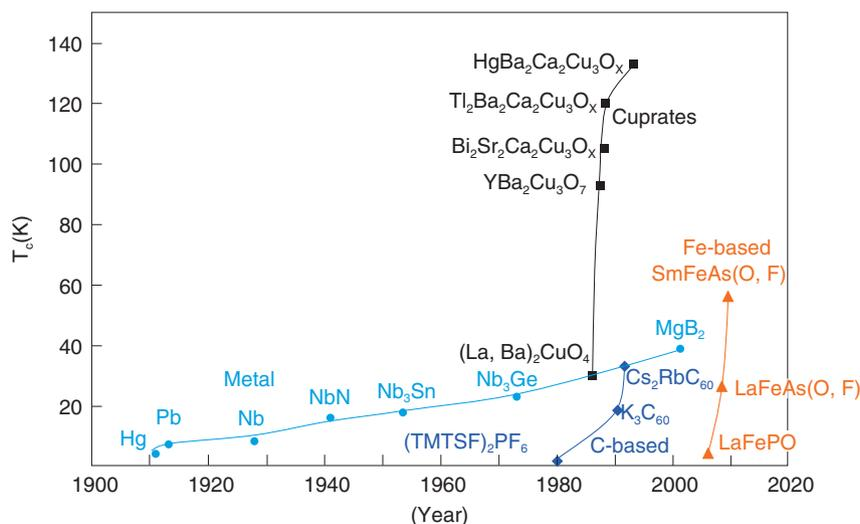
Fig. 2.  $T_c$  and discovery year of superconductors.
