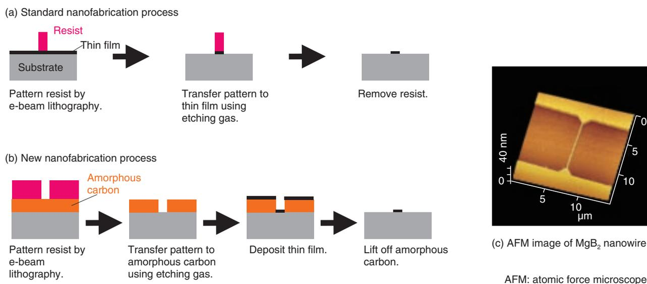
Fig. 3. Nanofabrication processes and MgB<sub>2</sub> nanowire.
