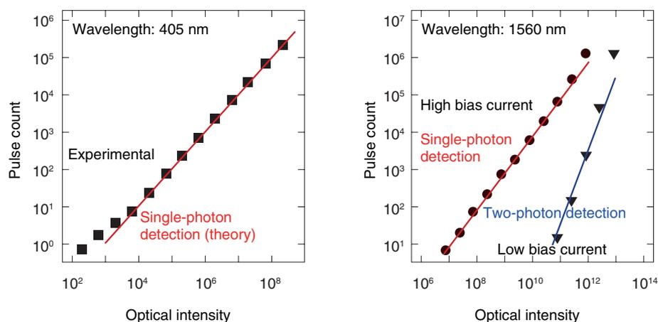
Fig. 4. Photon detection properties of MgB<sub>2</sub> nanowire.
