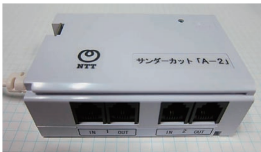
Photo 1. Lightning protection adaptor for analog port.
