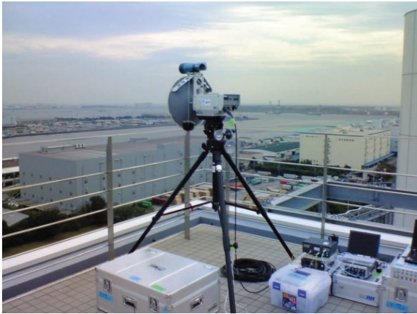
Fig. 2. Photograph of experiment on 5.8-km 10GbE transmission using forward error correction.
