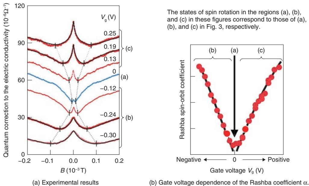
Fig. 6. Measurement of weak localization and weak antilocalization.
