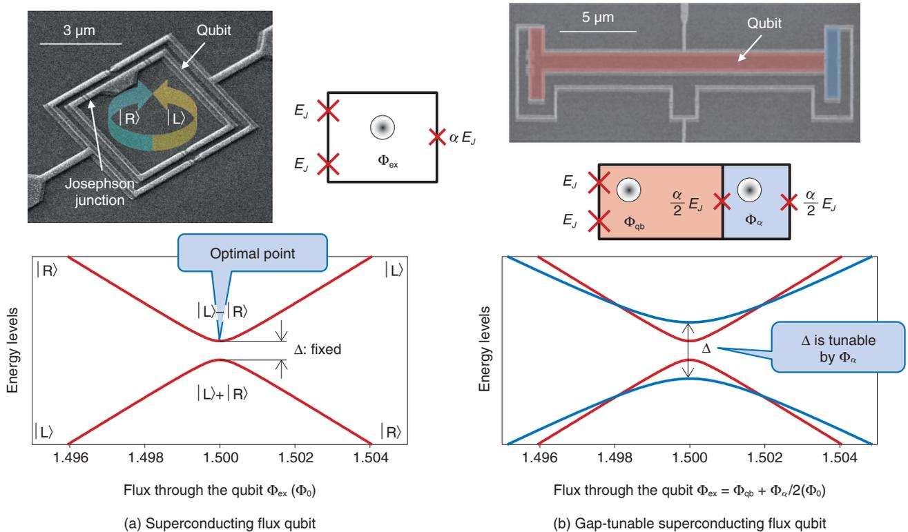
Fig. 4. Superconducting flux qubits and their energy levels.
