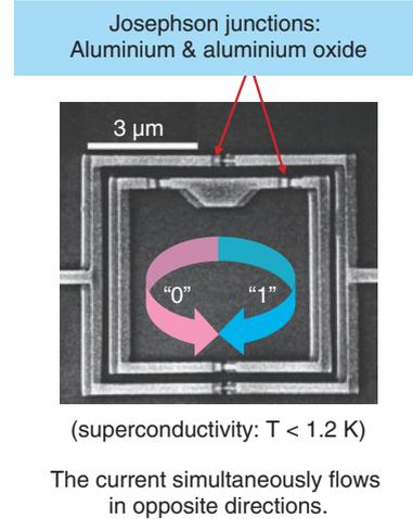
Fig. 2. Superconducting qubit.
