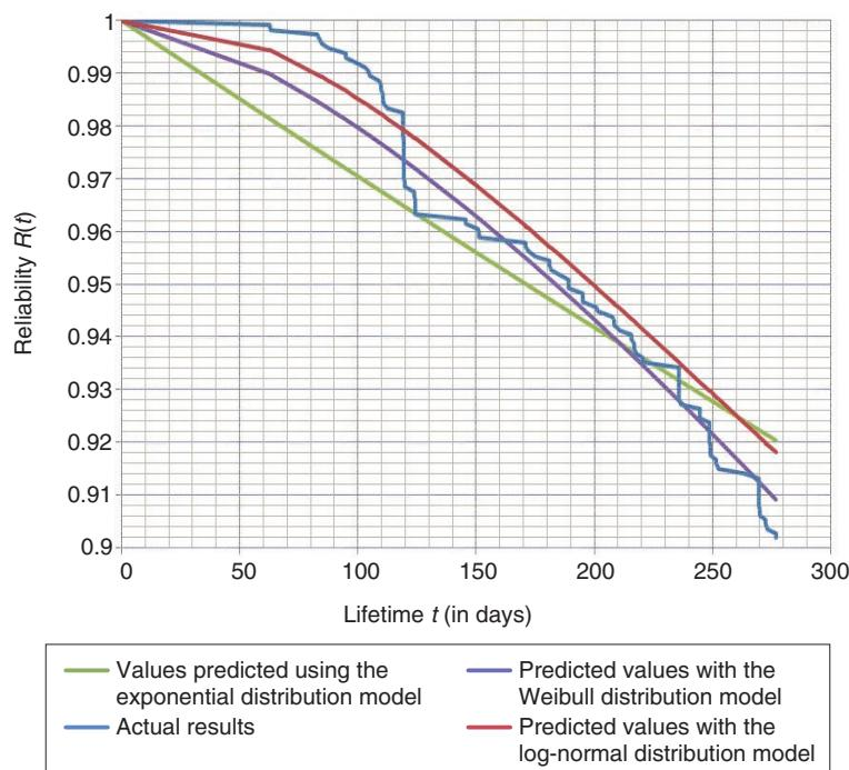
**Fig. 2.** HDD reliability calculated with lifetime distribution models.
