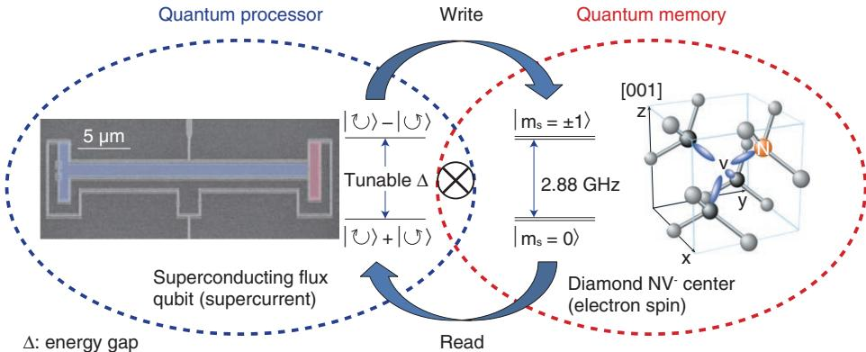
Fig. 2. Superconductor-diamond hybrid system.
