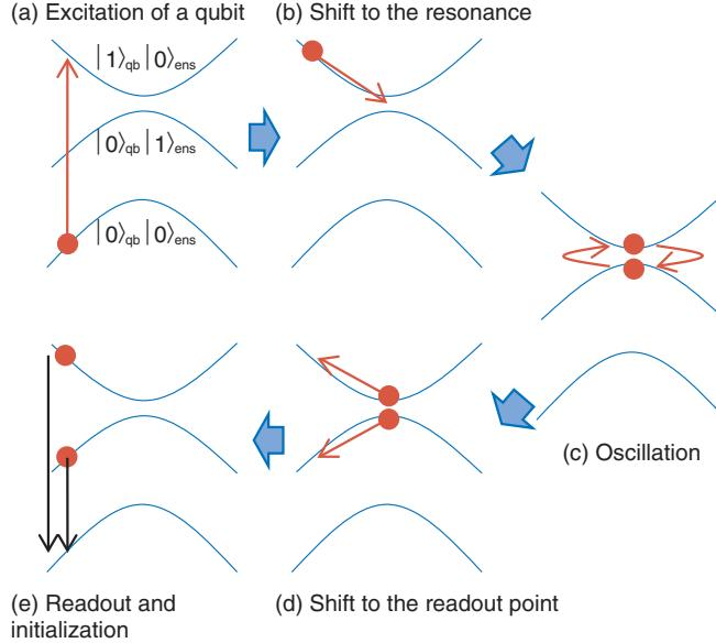
Fig. 7. Measurement sequence for observing vacuum Rabi oscillation.
