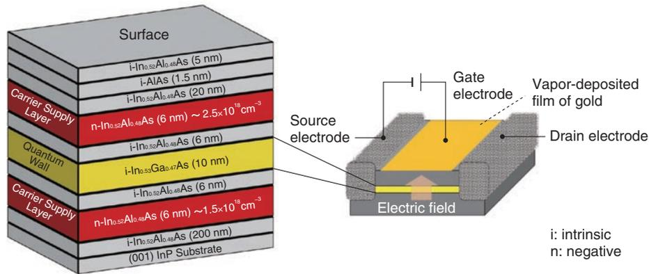
Fig. 4. Experimental sample and FET structure.
