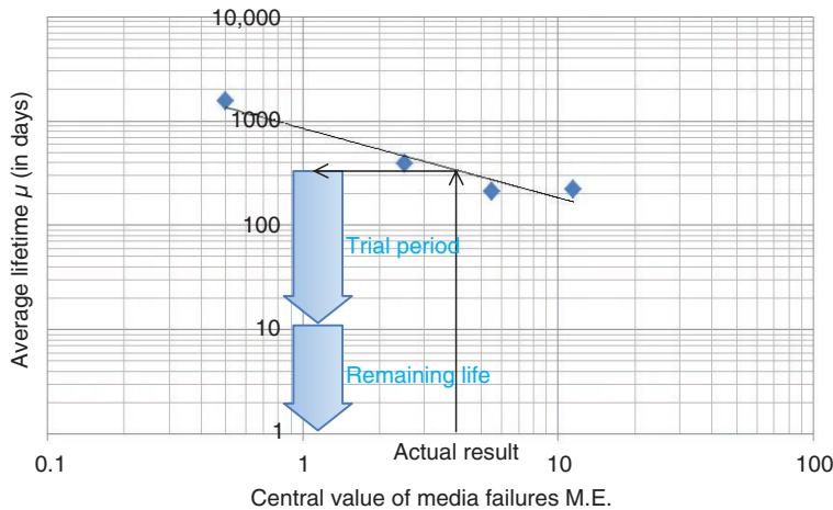
Fig. 7. Estimation of remaining life of an HDD.
