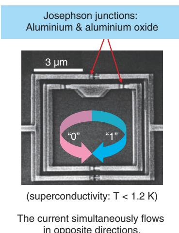
Fig. 2. Superconducting qubit.
