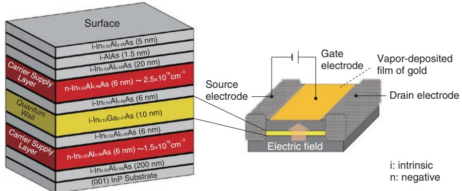
Fig. 4. Experimental sample and FET structure.
