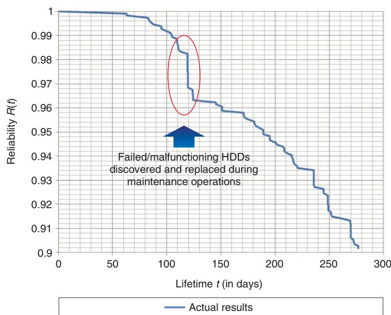
Fig. 1. HDD reliability calculated from failure statistics.
