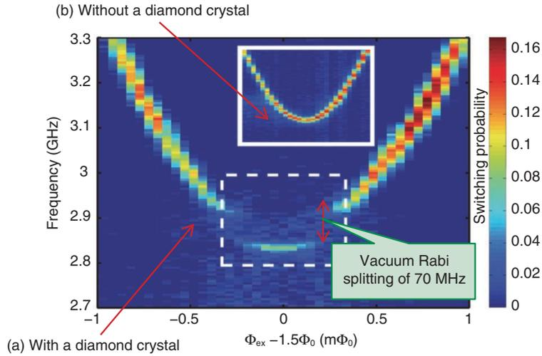
Fig. 6. Spectra of a superconducting flux qubit.
