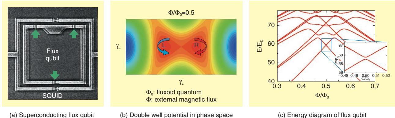
Fig. 2. Superconducting flux qubit as an artificial atom.
