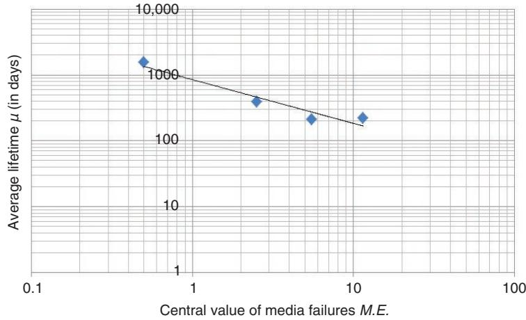
Fig. 5. Correlation between media failures and average lifetime.
