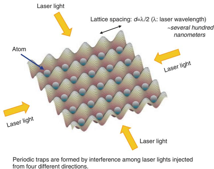
Fig. 4 Schematic illustration of optical lattice.
