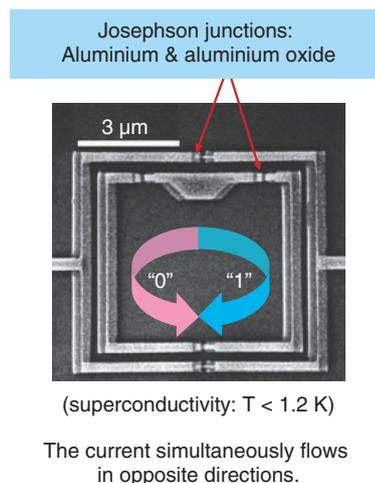
Fig. 2. Superconducting qubit.
