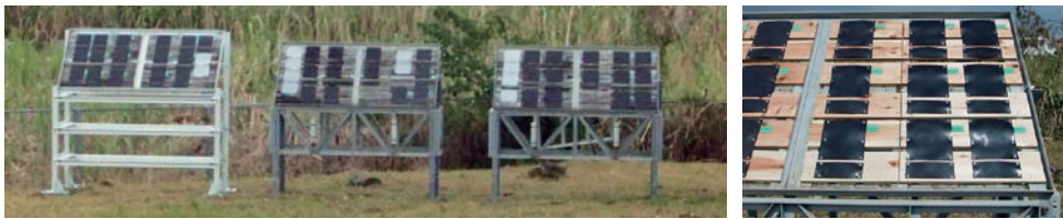
Fig. 1. Recycled PE samples set up at an outdoor exposure site. The magnified view on the right shows sheen remaining.
