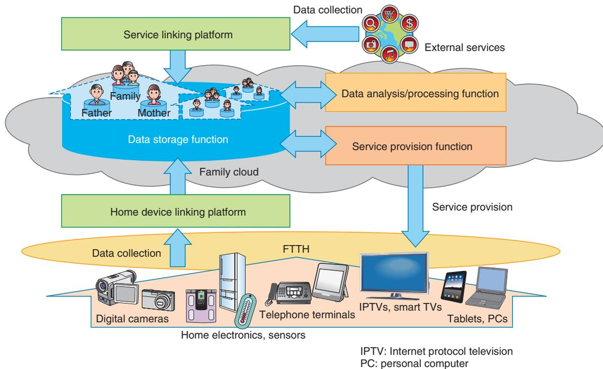
Fig. 1. SDH service architecture.
