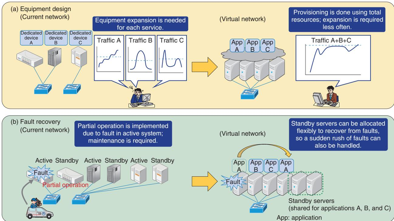
Fig. 2. Reducing OPEX with virtual networks.
