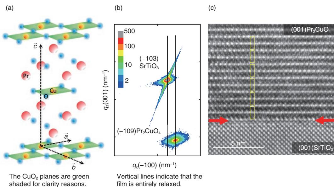
Fig. 1. (a) Crystal structure of  $\text{Pr}_2\text{CuO}_4$ , (b) high-resolution reciprocal space map of  $\text{Pr}_2\text{CuO}_4$  grown on (001)  $\text{SrTiO}_3$  substrate, and (c) high-resolution transmission electron microscopy image of  $\text{Pr}_2\text{CuO}_4$  grown on (001)  $\text{SrTiO}_3$  substrate taken at the interface.
