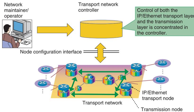
Fig. 6. Transport network architecture applying centralized transport control.
