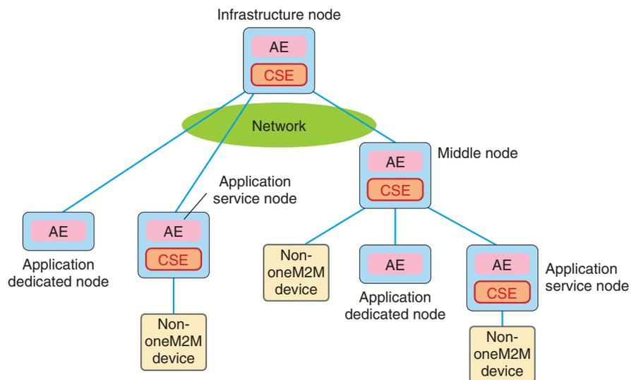
Fig. 4. Example structure of nodes and network.
