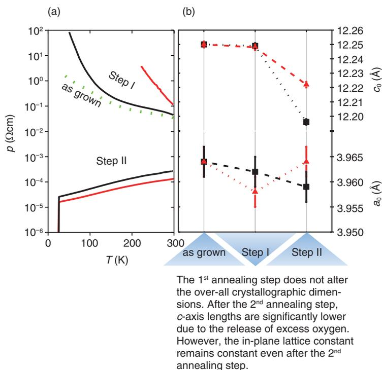
Fig. 5. (a) Temperature dependence of resistivity of  $\text{Pr}_2\text{CuO}_4$  thin films in as-grown state (green dashed line), after the 1<sup>st</sup> annealing step (step I), and after the 2<sup>nd</sup> annealing step (step II) and (b) trace of the crystallographic lattice parameters of  $\text{Pr}_2\text{CuO}_4$  thin films.
