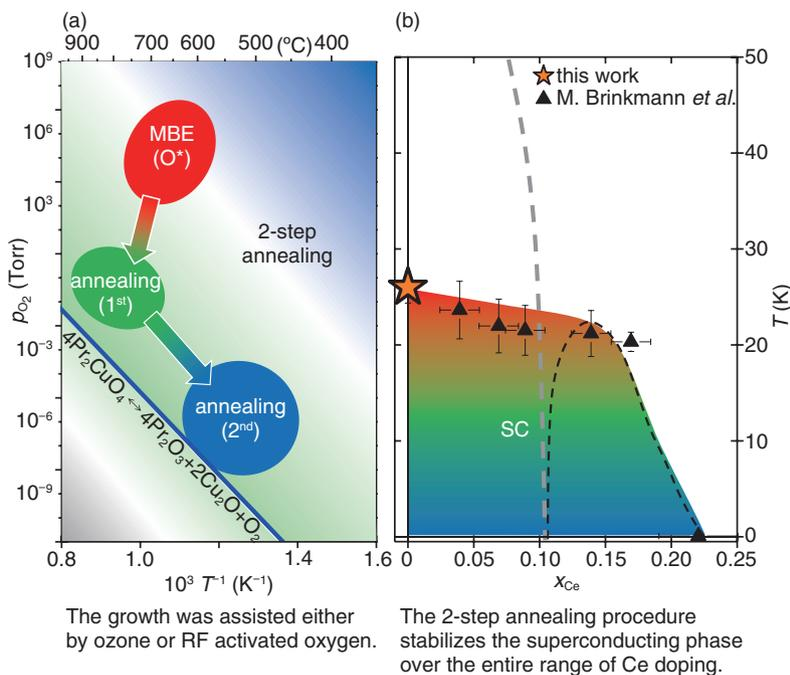
Fig. 4. (a) Thermodynamic phase diagram in the vicinity of the growth conditions of  $Pr_{2-x}Ce_xCuO_4$  (red area) and annealing conditions (green and blue area) and (b) superconducting phase diagram of  $Pr_{2-x}Ce_xCuO_4$  grown on (001)  $SrTiO_3$  substrates as a result of the annealing procedure shown on the left. Data denoted by triangles are taken from Ref. [34].
