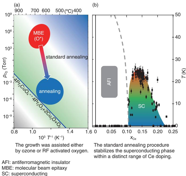
Fig. 3. (a) Thermodynamic phase diagram in the vicinity of the growth conditions of  $Pr_{2-x}Ce_xCuO_4$  (red area) and annealing conditions (blue area) and (b) superconducting phase diagram of  $Pr_{2-x}Ce_xCuO_4$  grown on (001)  $SrTiO_3$  substrates as a result of the annealing procedure shown on the left.
