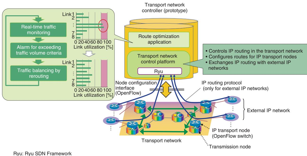
Fig. 7. Network architecture used in concept demonstration.
