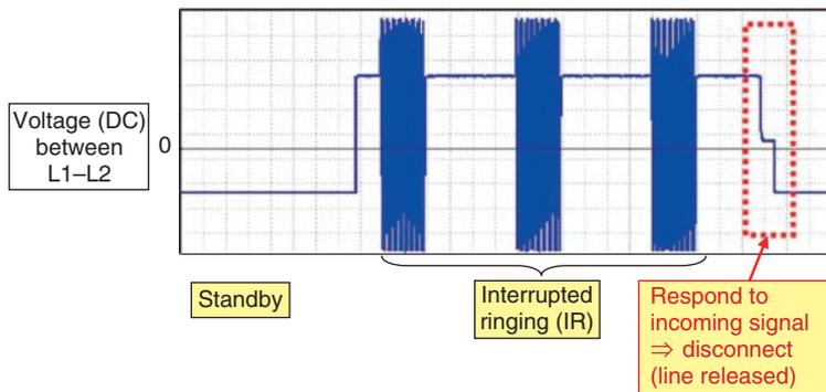
Fig. 5. Respond/disconnect waveform at time of incoming call.
