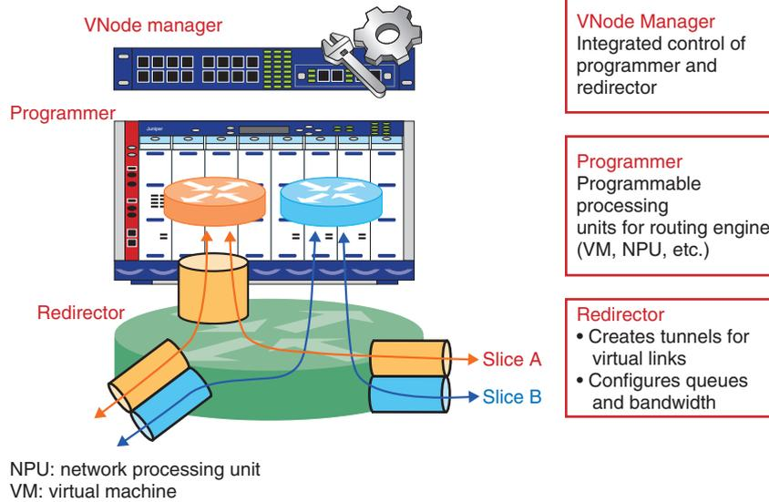
Fig. 4. Basic components of VNode system.
