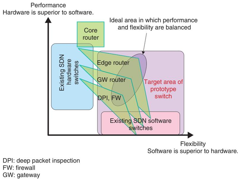
Fig. 2. Flexibility and performance target of Lagopus switch.
