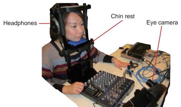
Fig. 3. Experimental setup to decode familiarity and preference for music from the eyes. Eye movements and pupillary responses of participant while she listens to a tune are measured using an eye camera.
