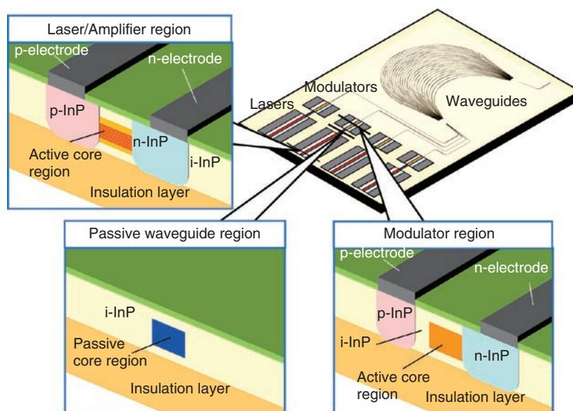
Fig. 1. Concept of PICs based on membrane optical devices.
