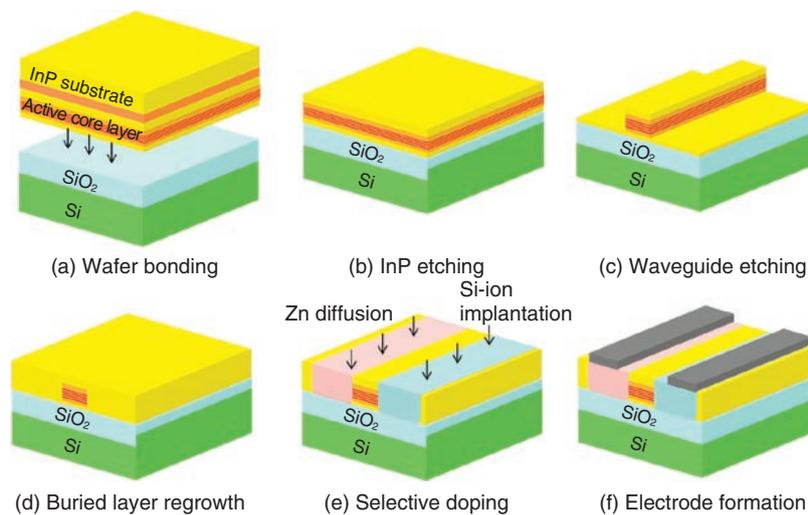
Fig. 3. PIC fabrication processes employing selective doping techniques.
