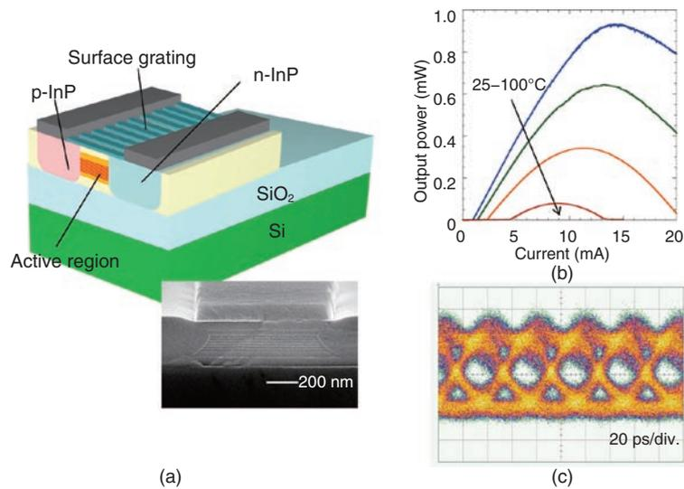
Fig. 5. (a) Device structure, (b) current-output characteristics, and (c) 25.8-Gbit/s modulating waveform of DFB laser on SiO<sub>2</sub>/Si.
