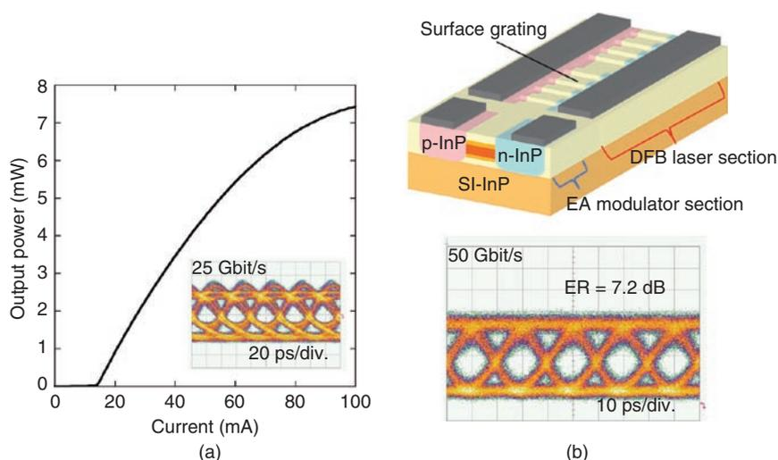
Fig. 4. Characteristics of membrane devices on InP: (a) directly modulated DFB laser, and (b) EA-DFB laser.
