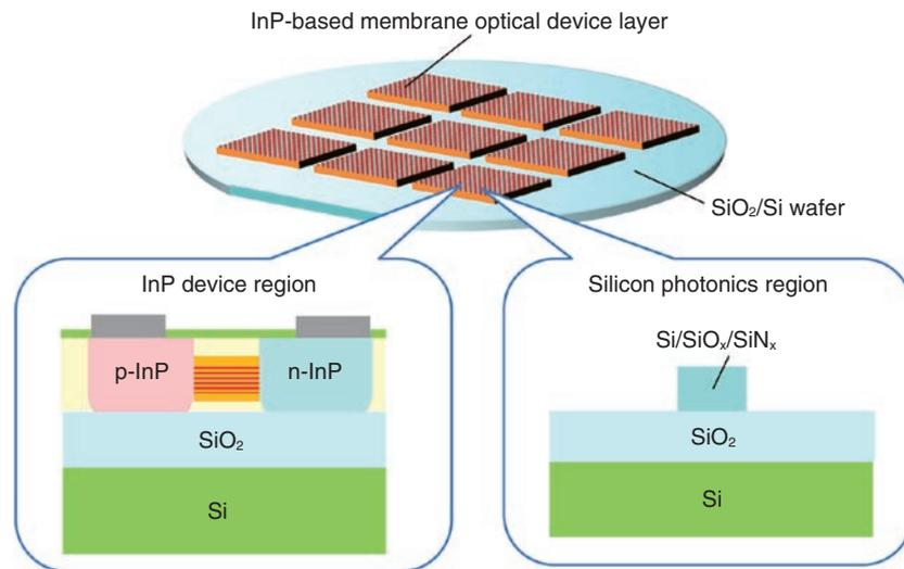
Fig. 2. Membrane optical devices integrated on silicon.
