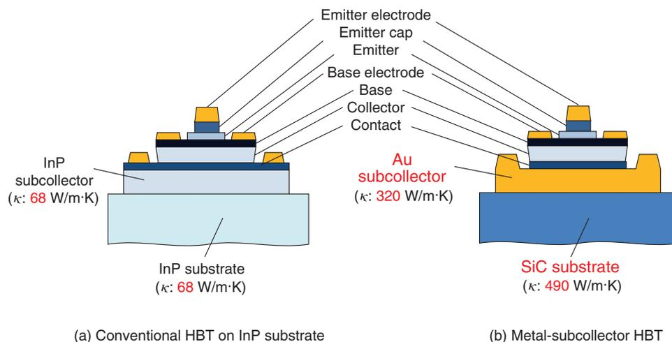
Fig. 1. Cross-sectional view of (a) conventional InP-based HBT on InP substrate and (b) metal-subcollector HBT on SiC substrate.
