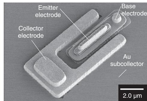
Fig. 4. Scanning electron microscope image of a fabricated metal-subcollector HBT with an emitter size of  $0.25 \mu\text{m} \times 4.0 \mu\text{m}$ .
