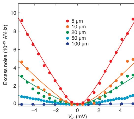
Fig. 4. Shot noise for different values of p-n junction length as a function of the bias applied to the electron channels  $V_{sd}$ .
