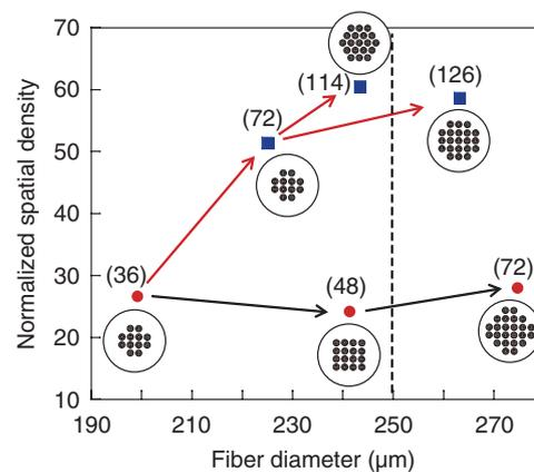
Fig. 6. Relationship between spatial density and fiber diameter of various multi-mode multi-core structures.
