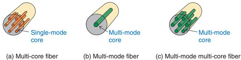
Fig. 2. Schematic diagram of multi-core and multi-mode fibers.
