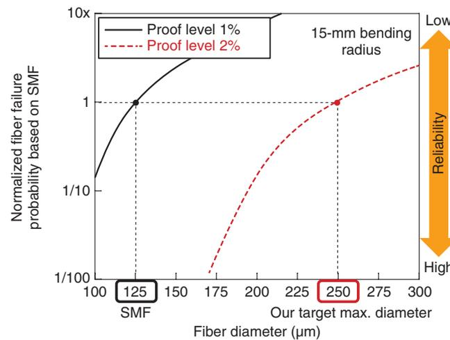
Fig. 5. Relationship between fiber failure probability and fiber diameter.
