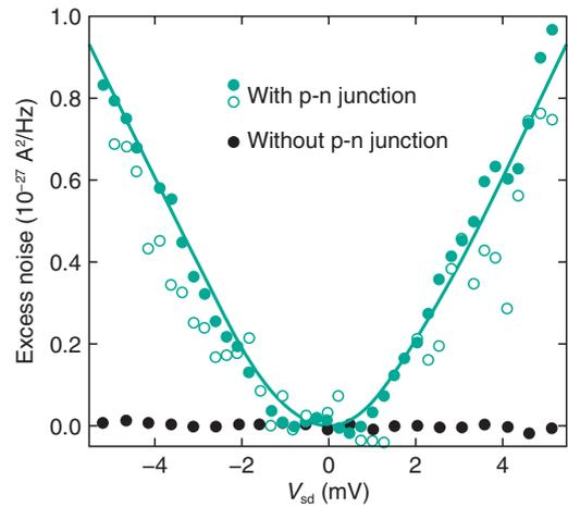
Fig. 3. Shot noise generated by p-n junction as a function of the bias applied to the electron channel  $V_{sd}$ . Solid cyan and black circles represent the measured noise in the presence and absence of p-n junctions. Open cyan circles represent the noise in the presence of a p-n junction obtained by applying bias to the hole channel.
