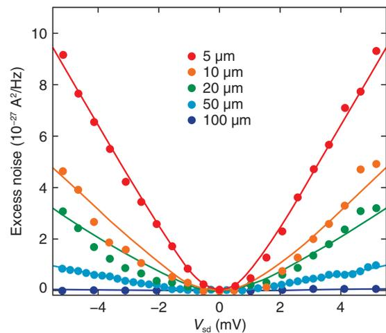
Fig. 4. Shot noise for different values of p-n junction length as a function of the bias applied to the electron channels  $V_{sd}$ .
