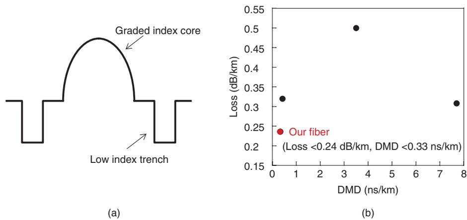
Fig. 7. (a) Schematic diagram of trench assisted graded-index core profile, (b) transmission loss vs. DMD of recently reported few-mode multi-core fibers.
