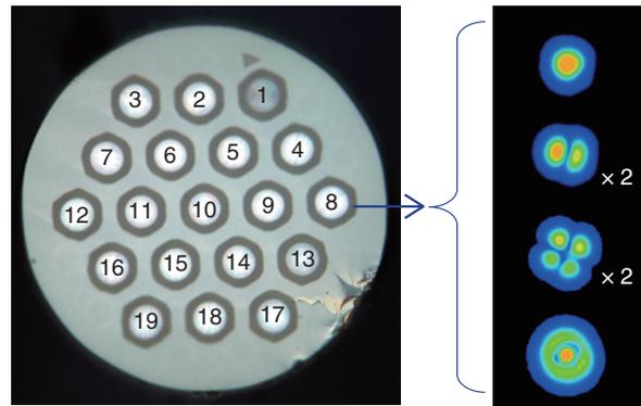
Six modes can propagate within each core.
