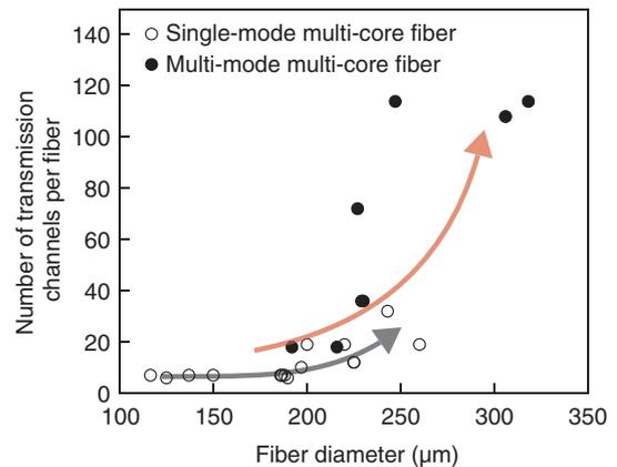
Fig. 3. Relationship between transmission channels per fiber and fiber diameter.
