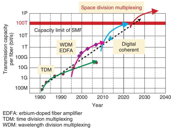
Fig. 1. Progress in transmission capacity per optical fiber.
