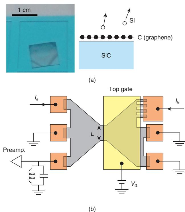
Fig. 2. ((a) left) Photograph of graphene grown on SiC. ((a) right) Schematic of graphene growth on SiC. (b) Device structure of graphene with a p-n junction. Gray region represents n-doped graphene. Tuning the bias of the top gate (yellow region) changes the carrier type in the gated region to a hole, and a p-n junction is formed at the interface between the gated and ungated regions. Orange regions are ohmic contacts.
