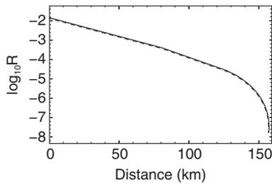
Fig. 2. Distance dependency of  $R$  of our scheme on a log scale. Here also, the solid, dashed, and dotted lines respectively represent cases with perfect phase modulation, a 3.6-degree modulation error, and a 7.2-degree modulation error.
