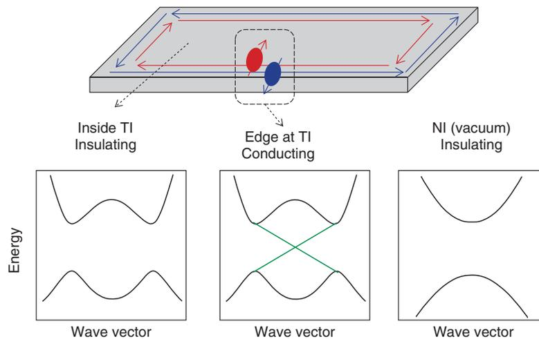
Fig. 1. Schematic energy dispersion of a topological insulator. TIs have different topology than normal insulators (including vacuum). Therefore, the band gaps must close at the interface between a TI and NI, resulting in conducting edge states.
