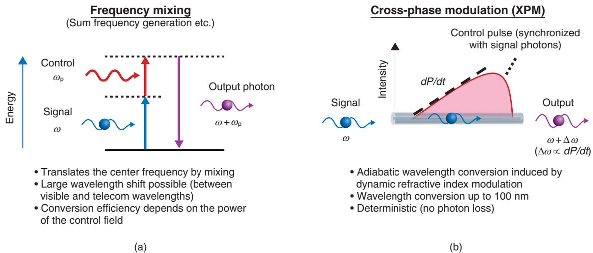
Fig. 2. Nonlinear optical effects for single-photon wavelength conversion.
