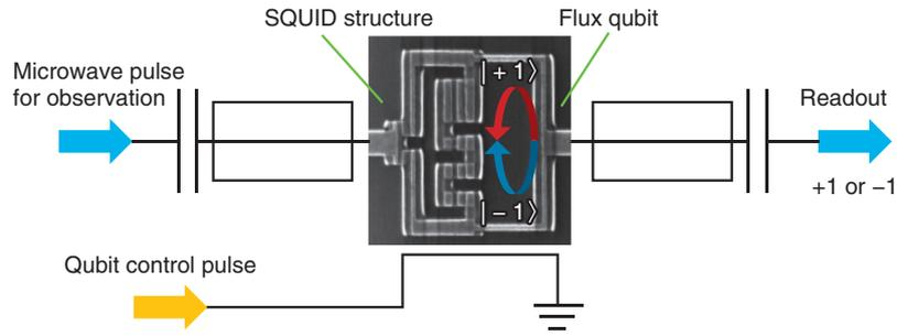
Fig. 2. Readout and control of superconducting flux qubit.
