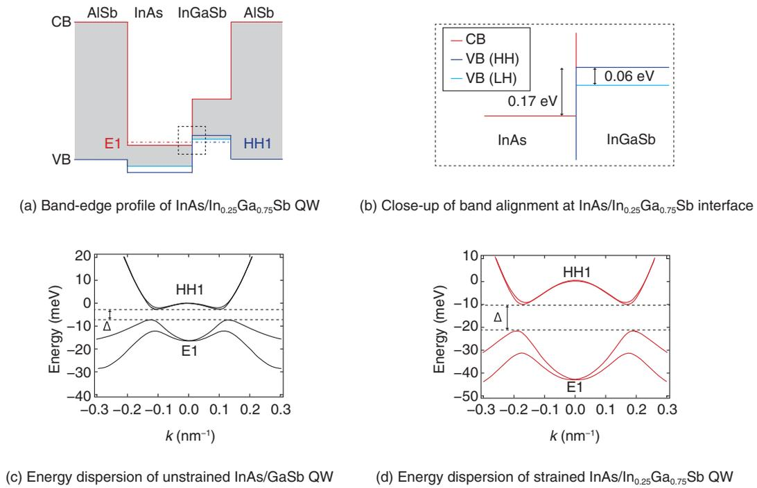
Fig. 2. Band structures of InAs/(In)GaSb QWs.
