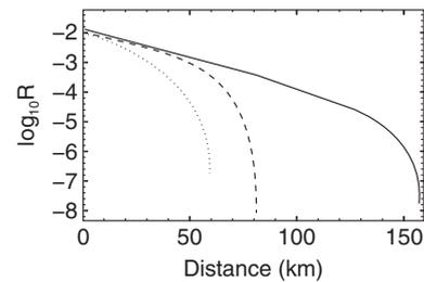
Fig. 1. Distance dependency of communication speed ( $R$ ) on a log scale. Solid, dashed, and dotted lines respectively represent cases with perfect phase modulation, a 3.6-degree modulation error, and a 7.2-degree modulation error.
