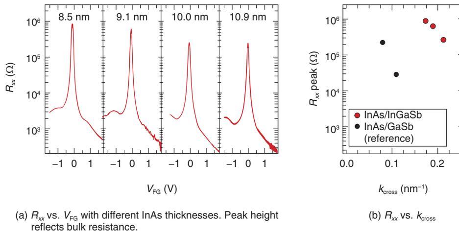
Fig. 5. Demonstration of high bulk resistance in deep band inverted regime.
