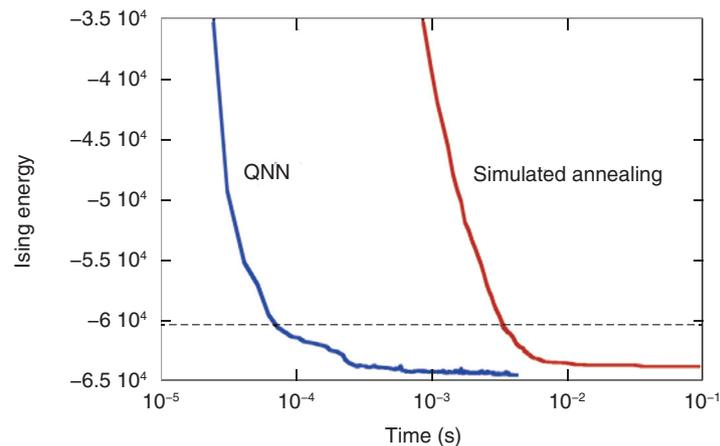
The blue and red curves show the energies obtained with the QNN and simulated annealing run on a CPU. The dotted line denotes the reference energy obtained with an algorithm called GW-SDP. It took 3.2 ms to reach the reference energy using simulated annealing, while the QNN delivered the solution with the same Ising energy in only 0.7 ms.
