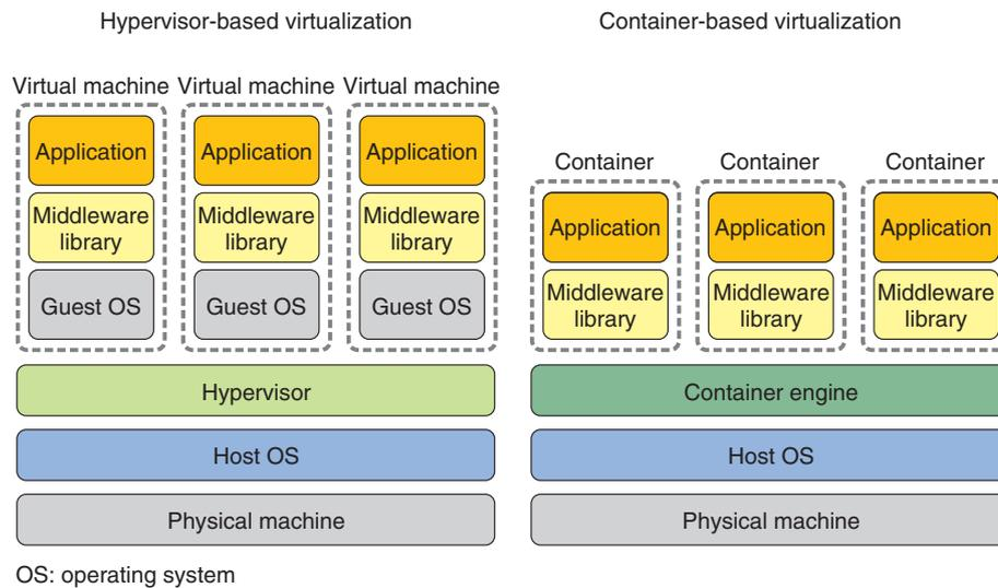
Fig. 3. Schematic of hypervisor-based virtualization and container-based virtualization.
