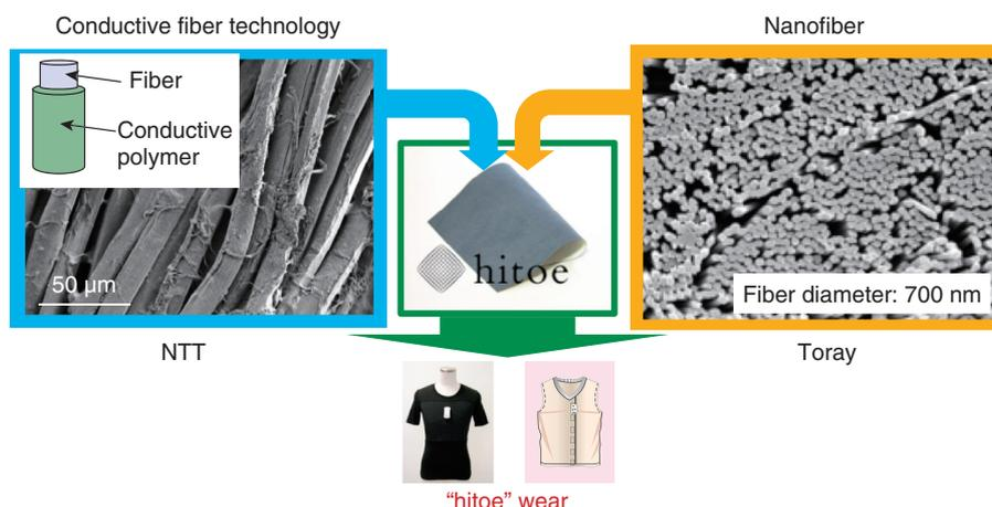
Fig. 1. Cross-industry collaboration with Toray to develop “hitoe.”
