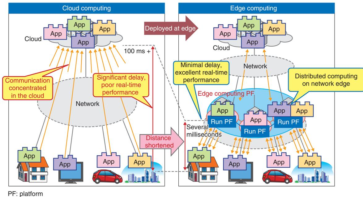
Fig. 2. Comparison of cloud computing and edge computing.
