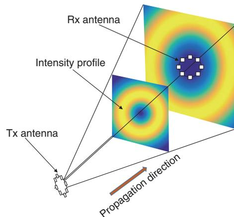
Fig. 3. Conceptual drawing of OAM beam divergence.
