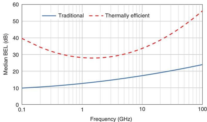
Fig. 6. BEL calculation result example in new Recommendation ITU-R P.[BEL].
