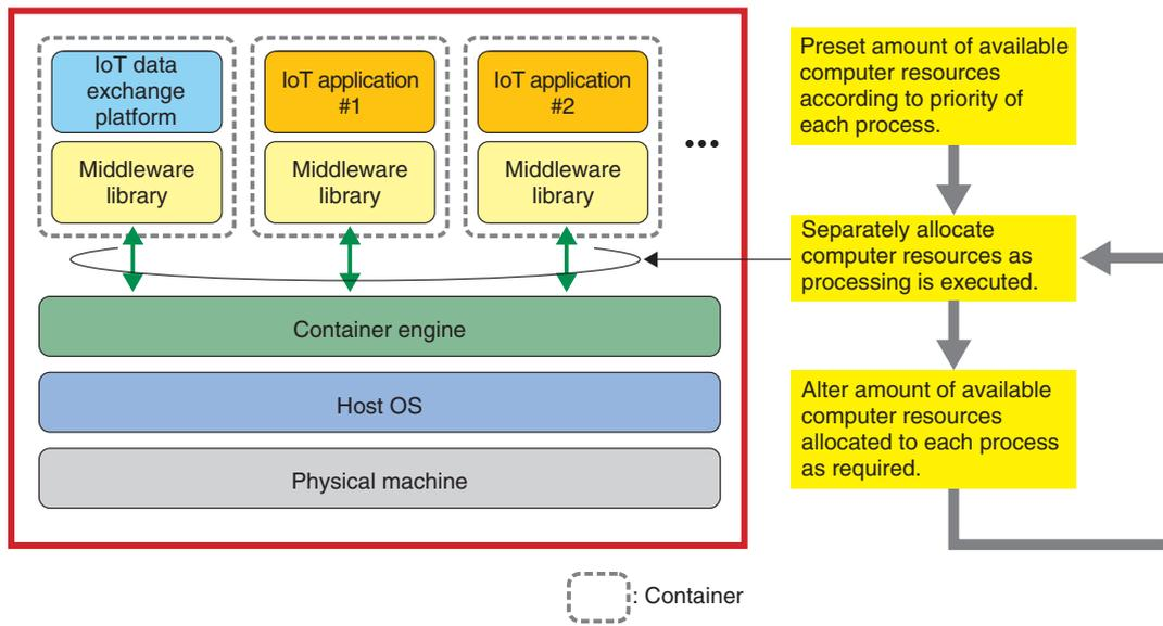
Fig. 4. Schematic of edge server using container-based virtualization.
