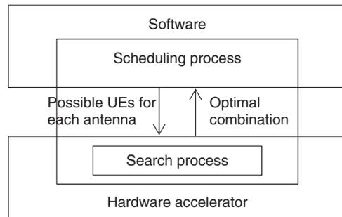
Fig. 4. Hardware acceleration for the scheduling process.
