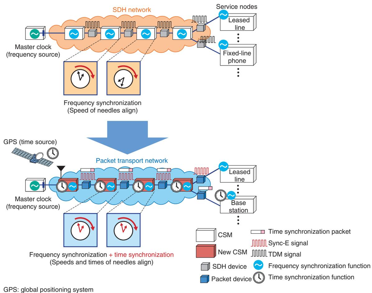
Fig. 1. Frequency/time synchronization using clock path network.
