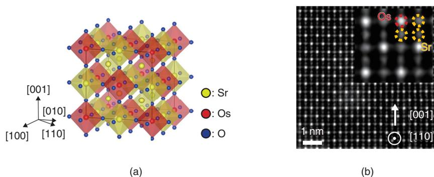
Fig. 1. (a) Schematic diagram of  $\text{Sr}_3\text{OsO}_6$  (double perovskite). The yellow, red, and blue spheres respectively indicate Sr, Os, and O atoms. (b) Atomic scale microscopy (scanning transmission electron microscopy) image of a  $\text{Sr}_3\text{OsO}_6$  film viewed along the  $[110]$  direction. We can clearly see the atomic ordering depicted in Fig. 1(a).
