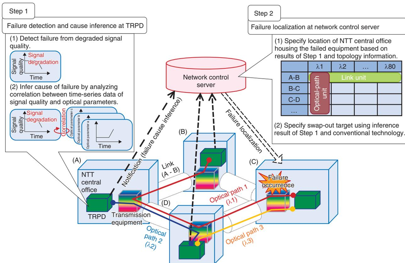
Fig. 1. Failure localization method.
