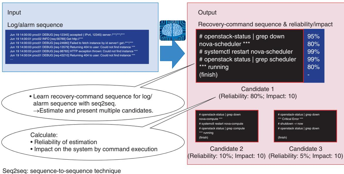
Fig. 1. Outline of automatic generation of recovery-command sequences.
