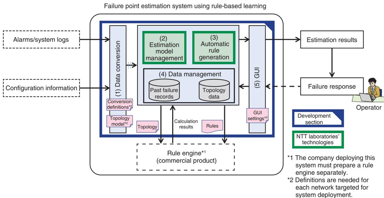
Fig. 2. Failure point estimation system using rule-based learning.
