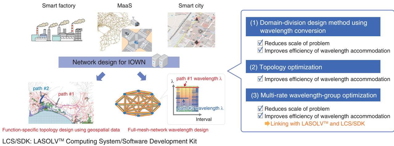
Fig. 2. Accommodation-design technology based on spatial data science.
