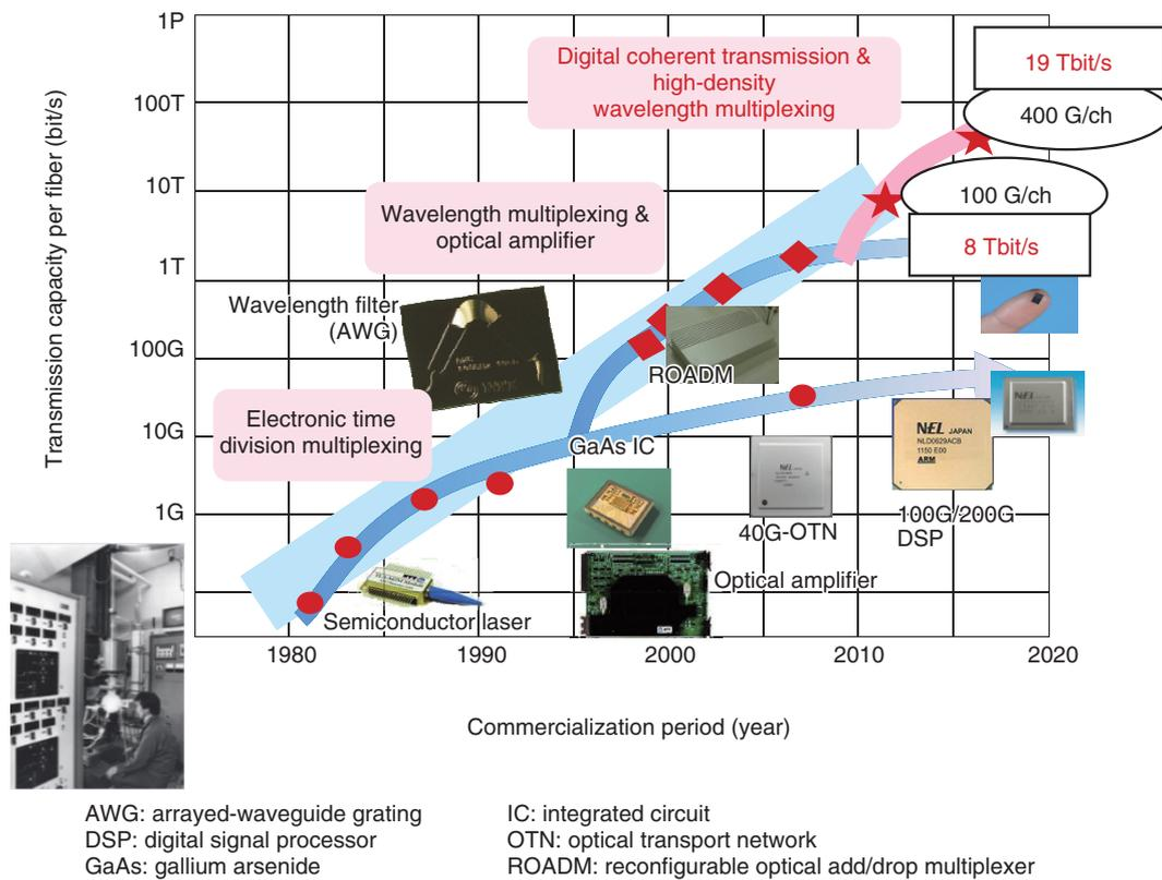
Fig. 2. Progress in photonics technology enabling traffic growth.
