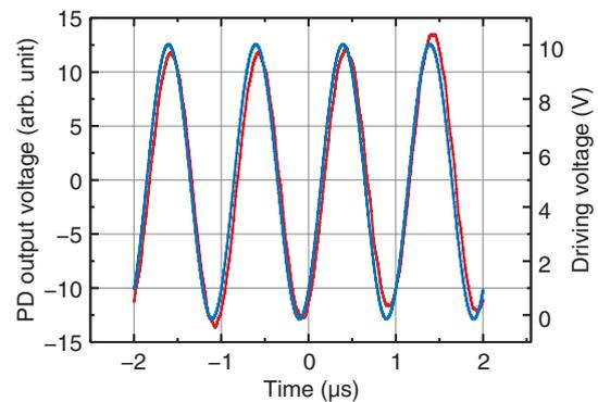
Fig. 6. Modulation characteristics of EO PM.
