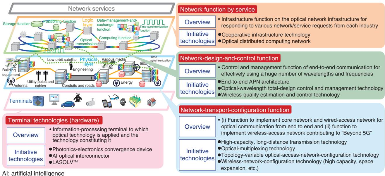
Fig. 1. Basic functions comprising the APN.
