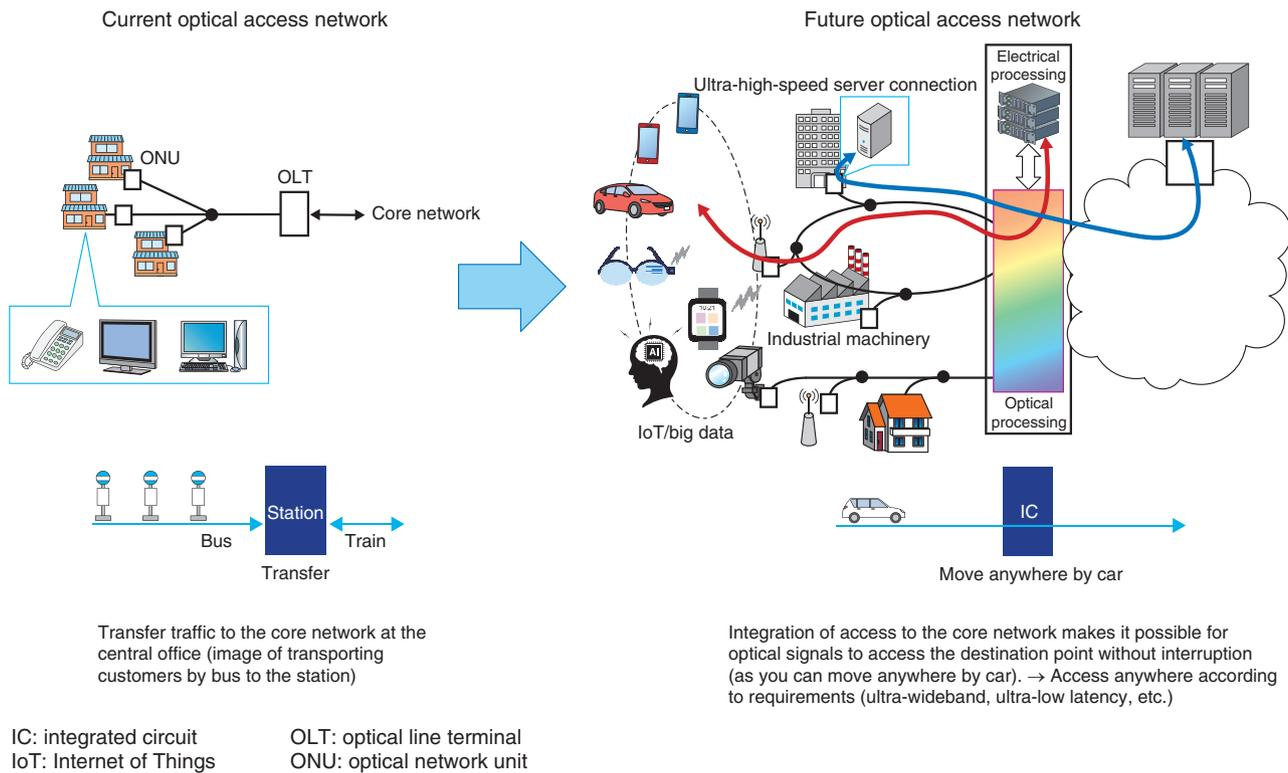
Fig. 1. Future image of optical access network.
