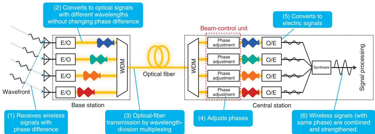
Fig. 3. Remote-beamforming technology (receiving side).
