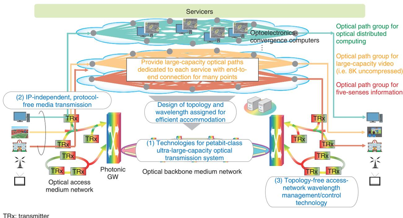
Fig. 1. Overview of optical full-mesh network.
