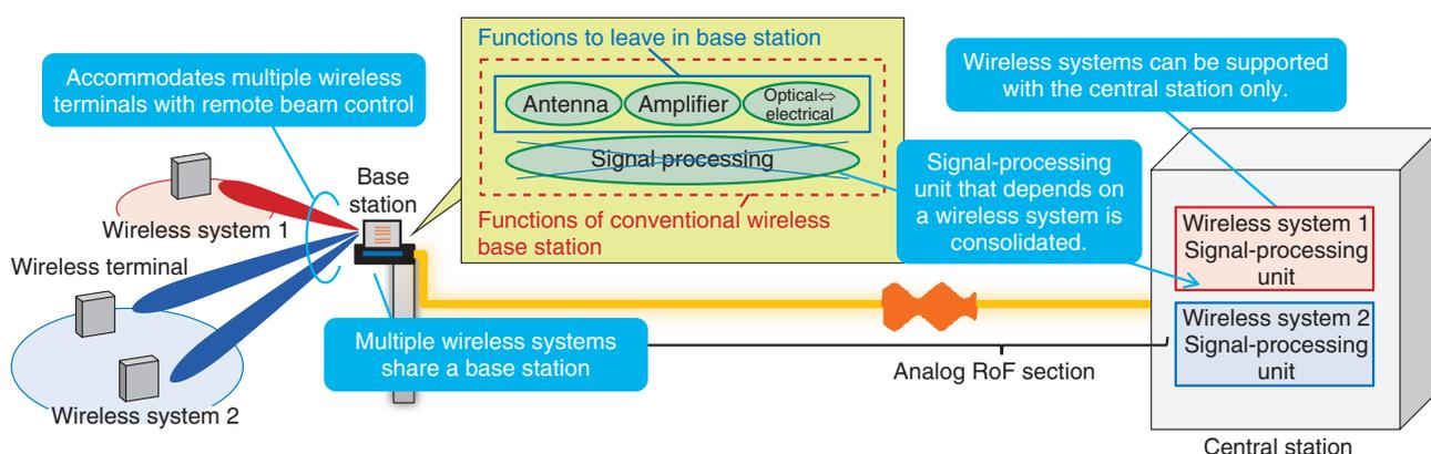
Fig. 2. Function consolidation by using analog RoF.
