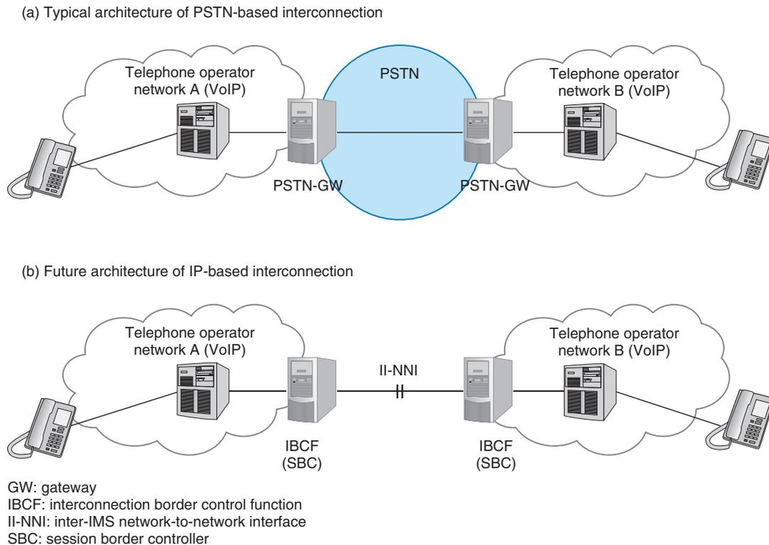
Fig. 1. Architecture of interconnection for VoIP services.
