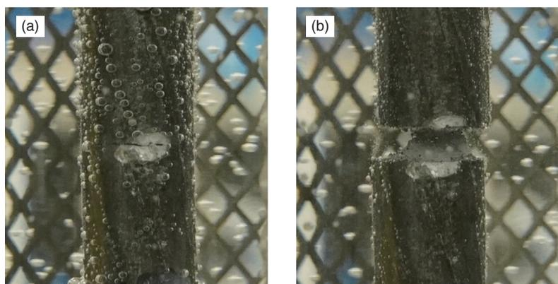
Fig. 1. Fracture of reinforcing steel bar from accelerated test of hydrogen embrittlement: (a) immediately before and (b) immediately after fracture.
