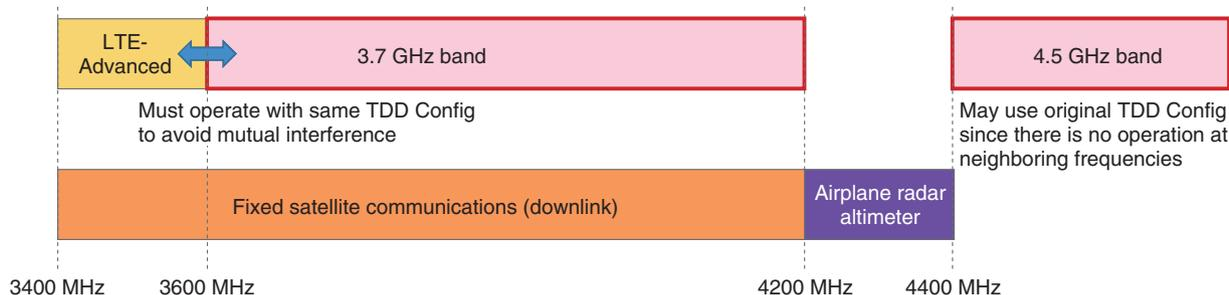
Fig. 1. Frequency allocation in 3.7 GHz band and relationship with LTE 3.5 GHz band.
