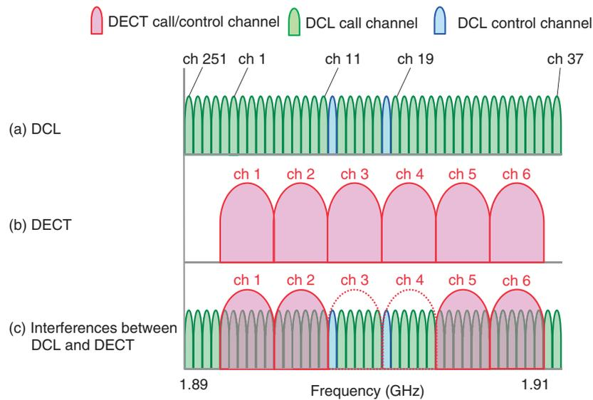
Fig. 1. Frequency allocation of the DCL and DECT.
