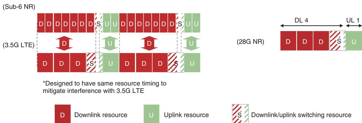
Fig. 2. TDD Config used in Japan's 5G frequencies.
