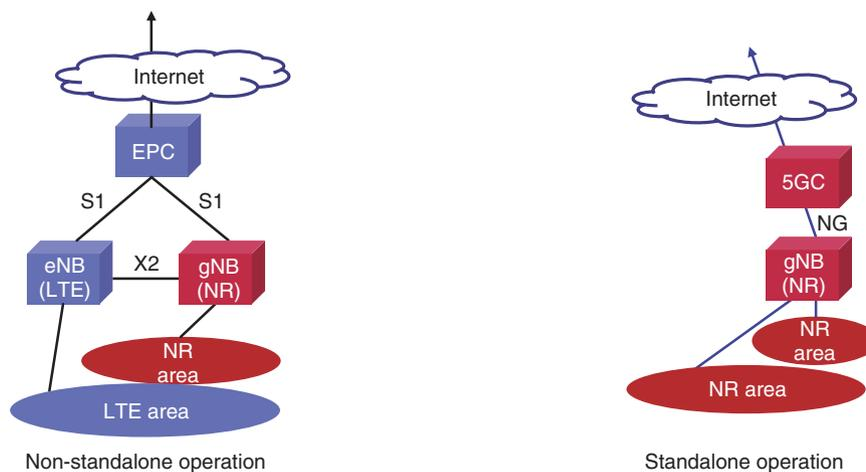
Fig. 5. Network configuration in 5G.
