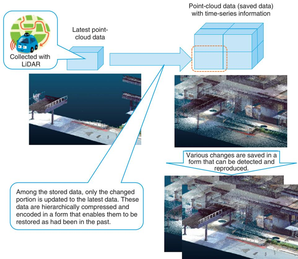
Fig. 4. Overview of 4D-point-cloud coding technology.
