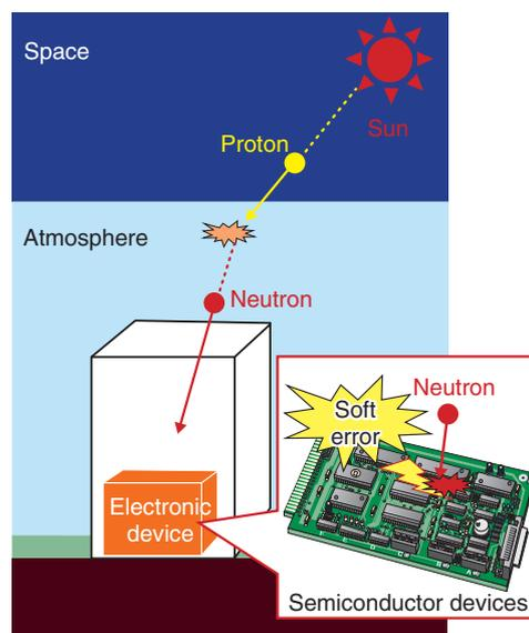
Fig. 3. Mechanism of soft error occurrence.
