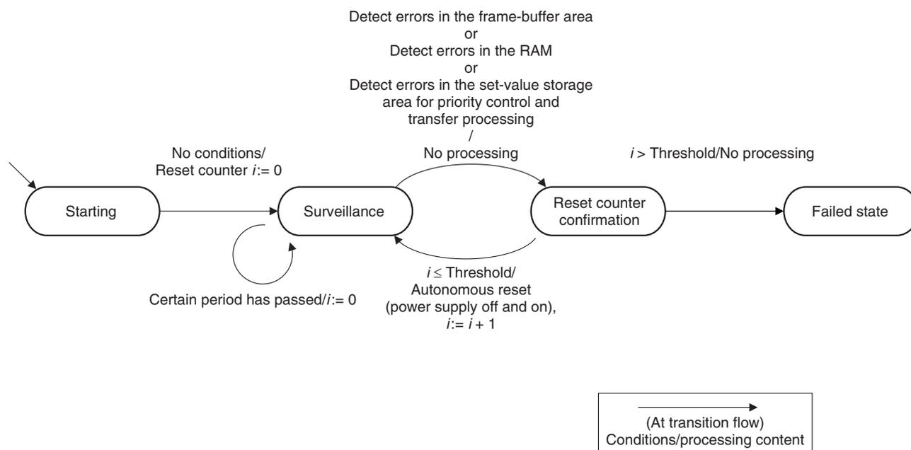
Fig. 5. Transition flow of the autonomous reset function.
