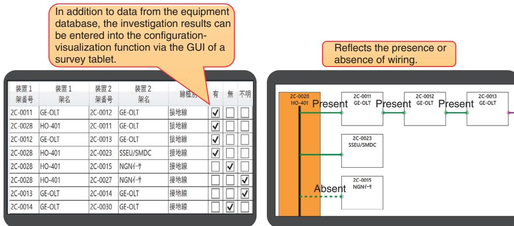
Fig. 3. Configuration-visualization function.
