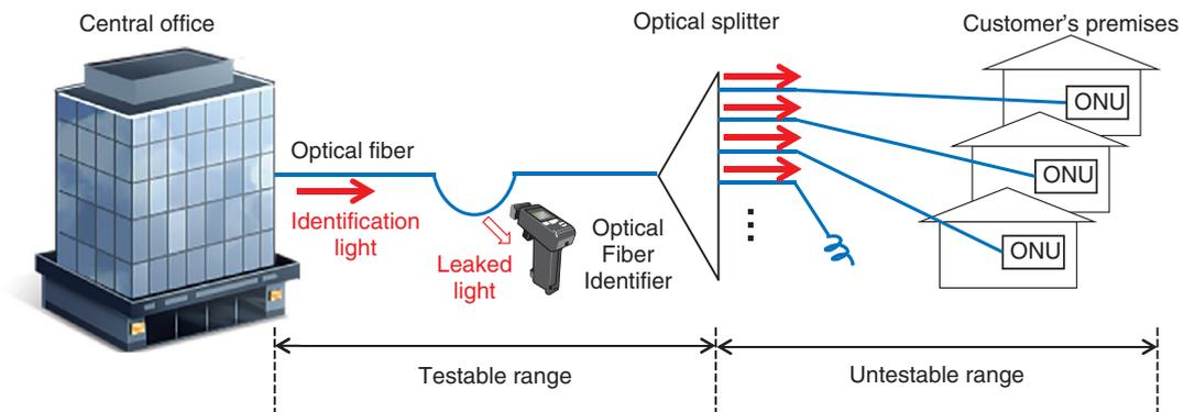
Fig. 1. Fiber identification in optical access networks.
