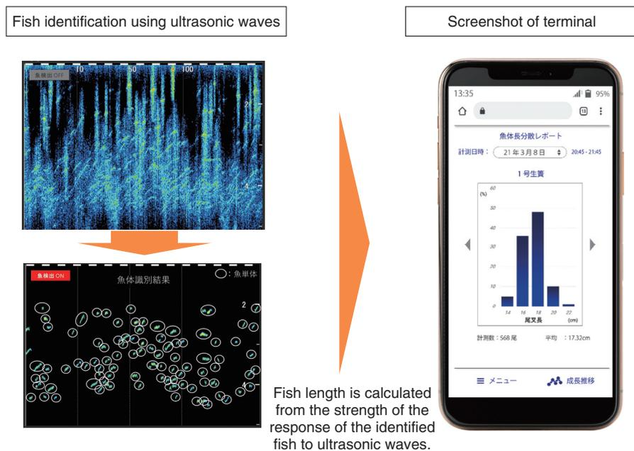
Fig. 2. Illustration of measuring fish length.
