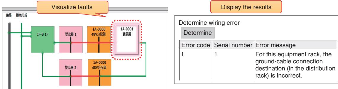
Fig. 4. Function for automatically determining the status of grounding configuration.
