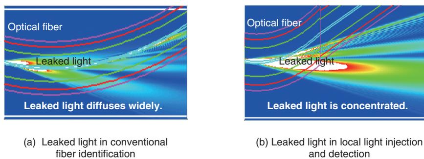
Fig. 3. Contour map of leaked light intensity.
