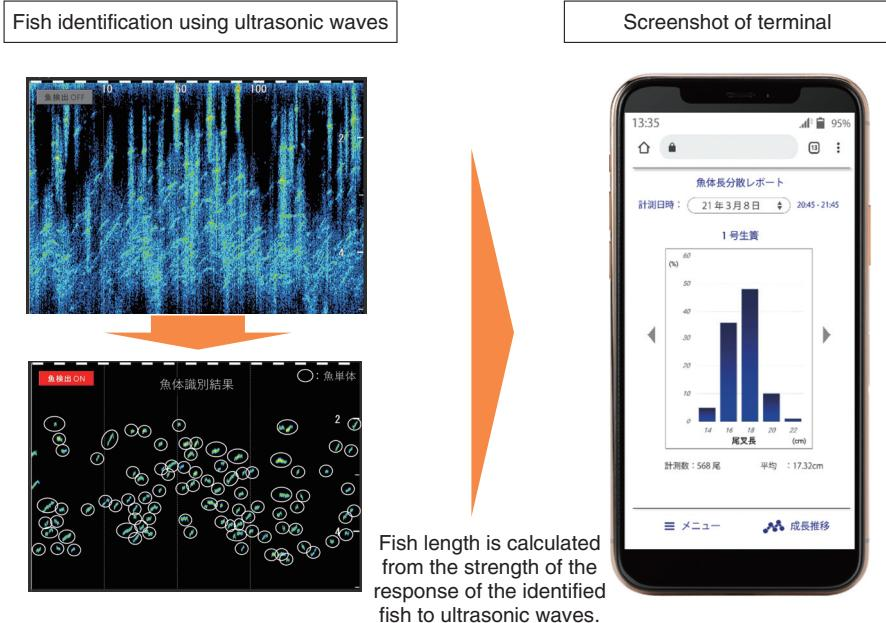
Fig. 2. Illustration of measuring fish length.
