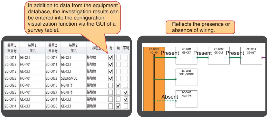
Fig. 3. Configuration-visualization function.
