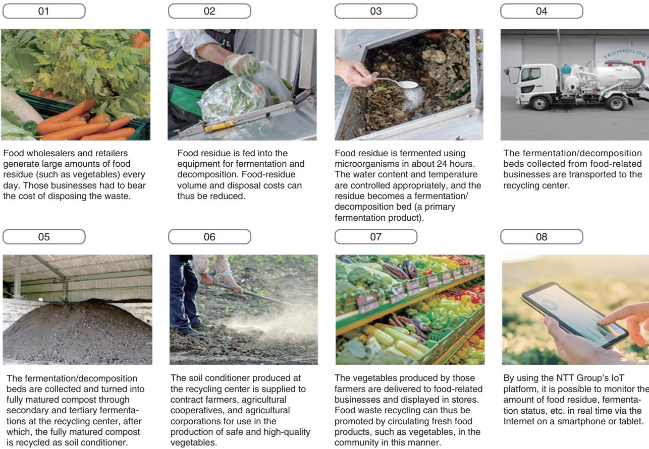
Fig. 2. The process of each solution.
