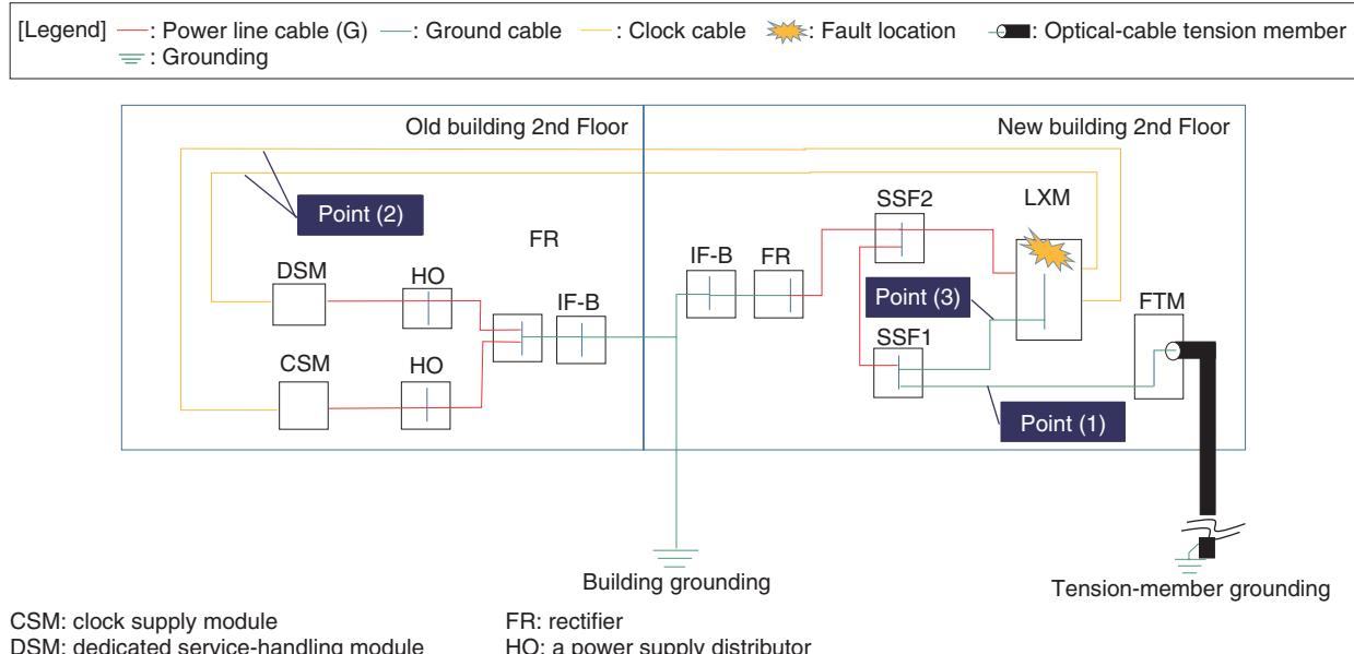
Fig. 5. On-site investigation of the building and identified configuration points.
