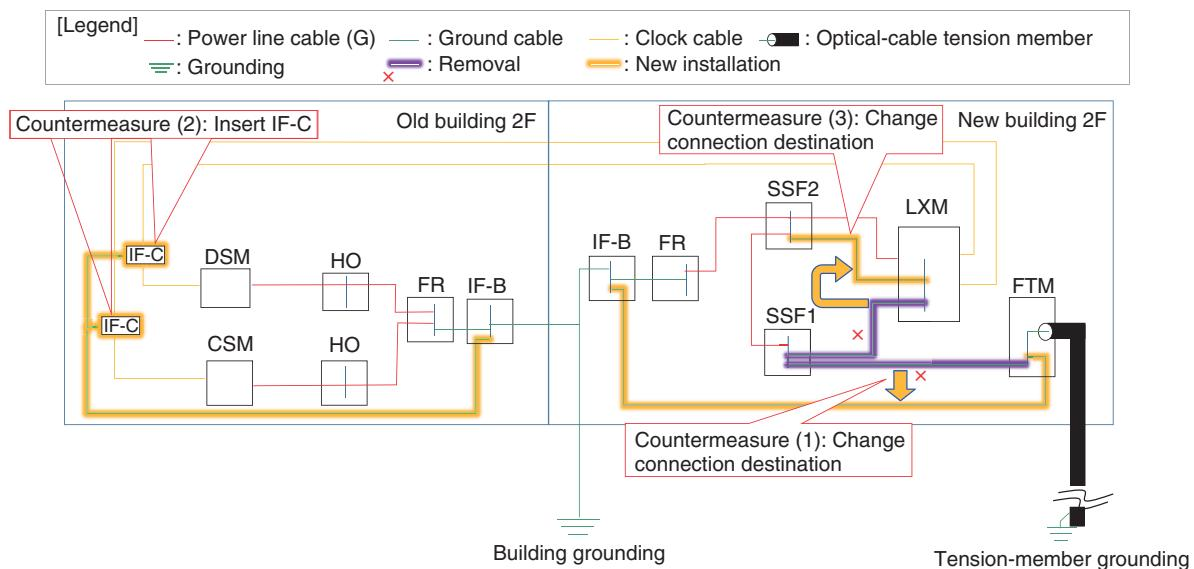
Fig. 9. The proposed lightning-damage countermeasures.
