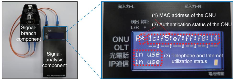
Fig. 5. Prototype of MAC address capture device and its display screen.
