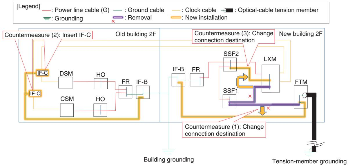
Fig. 9. The proposed lightning-damage countermeasures.
