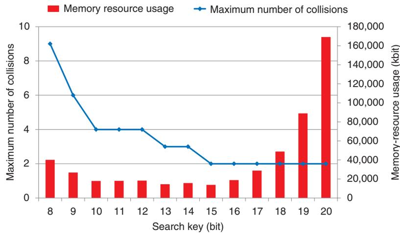
Fig. 8. Maximum number of output collisions when 500 random hash keys are input to the hash function using MurmurHash3 and memory-resource usage of the hash-based NTC.
