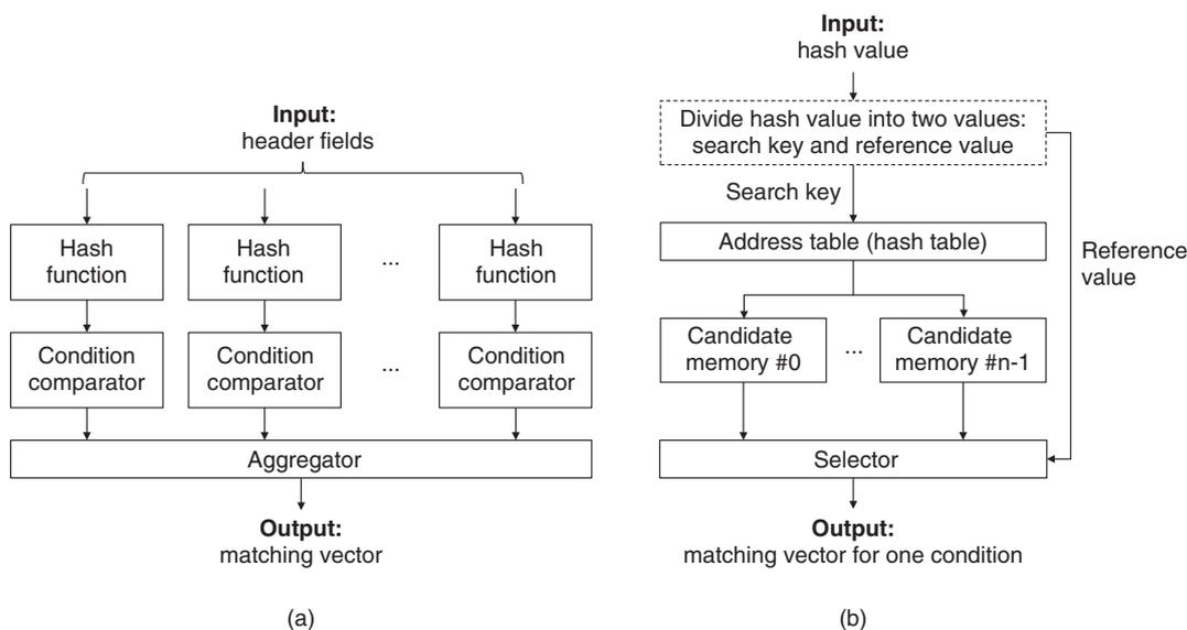
Fig. 7. Block diagrams of hash-based NTC: (a) overall architecture and (b) detailed condition comparator.
