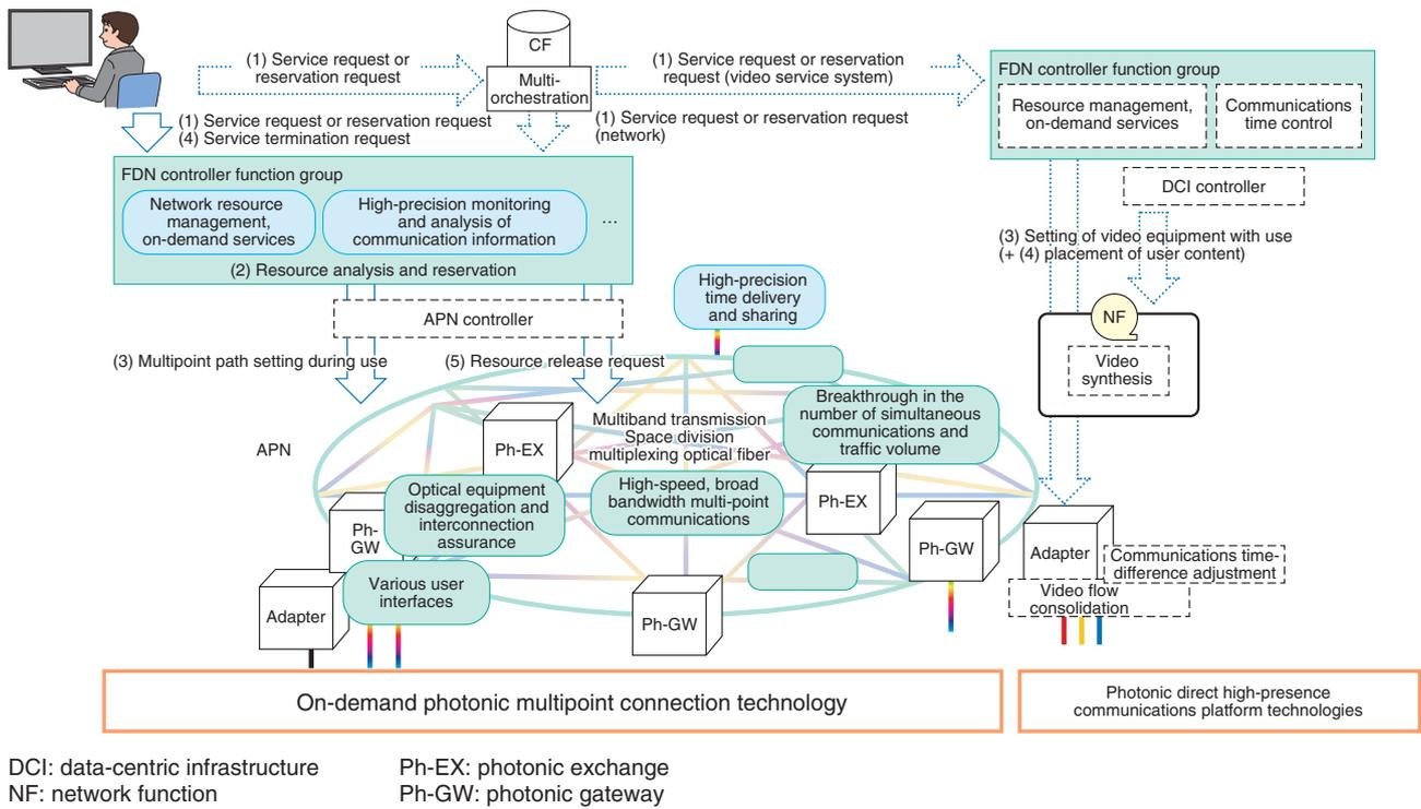
Fig. 3. On-demand photonic multipoint connection technology workflow.
