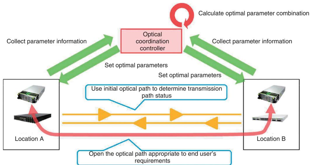
Fig. 2. Overview of automatic optical path provisioning technology.
