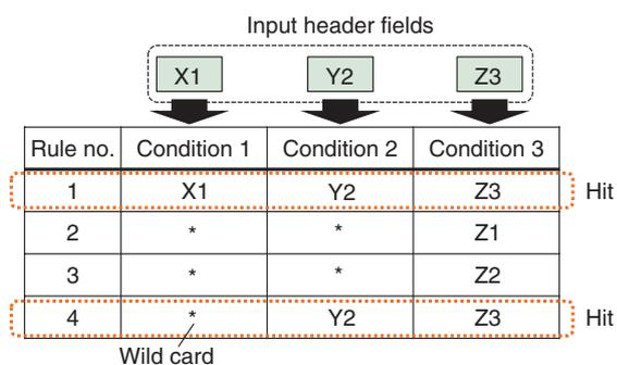
Fig. 3. Concept of NTC using partial match search.
