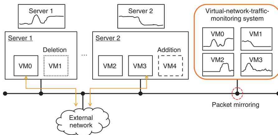
Fig. 1. Network-traffic monitoring using virtual-network-traffic-monitoring system.
