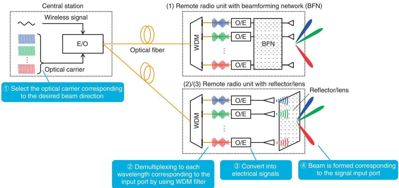
Fig. 3. Remote beamforming scheme using passive beamformer.
