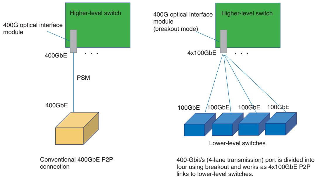
Fig. 4. Conventional P2P connection and breakout connection.
