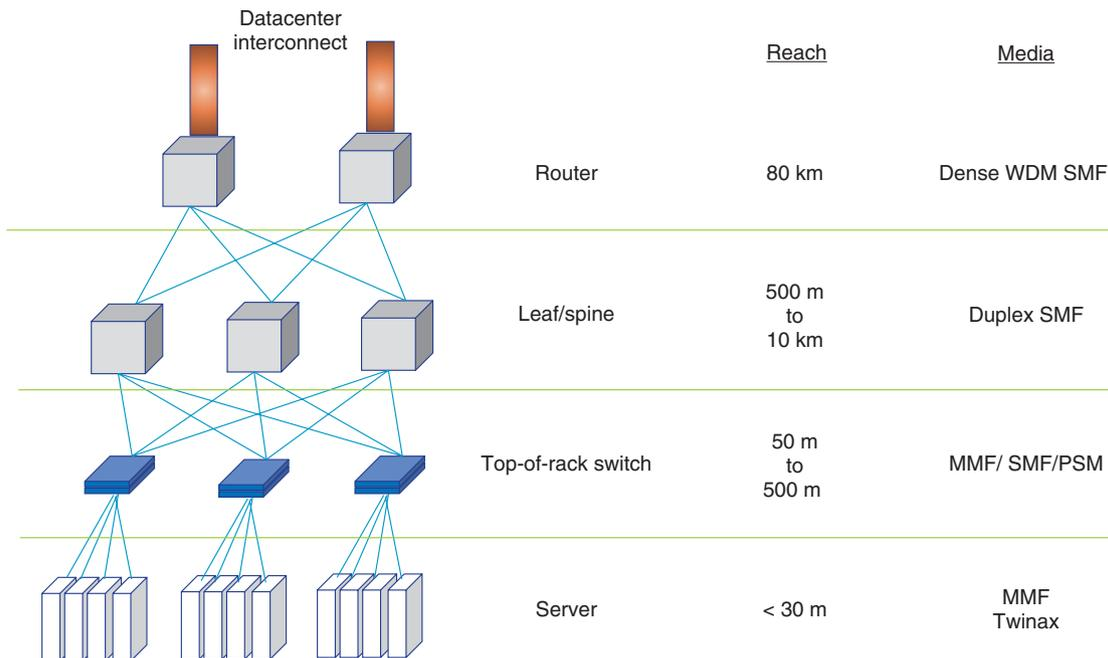
Fig. 2. Applications of P2P Ethernet interfaces (datacenter).
