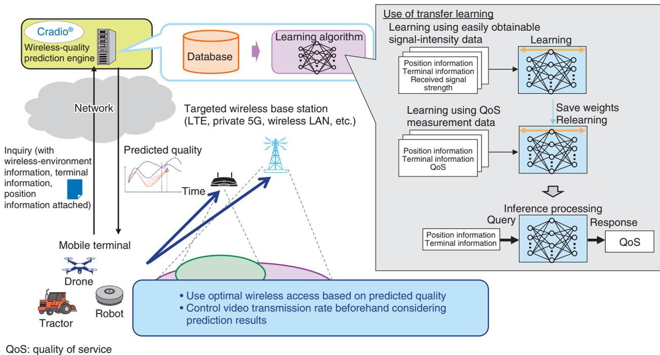
Fig. 4. Wireless-quality prediction/estimation technologies.
