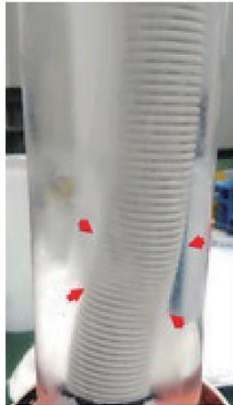
Fig. 6. Part of the PF pipe deformed due to concentrated stress.
