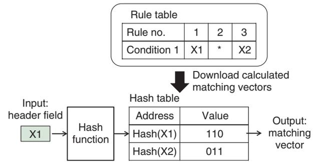
Fig. 6. Operation of hash-based NTC, which obtains a matching vector from the hash table. The matching vector is calculated in advance and downloaded to the hash table.
