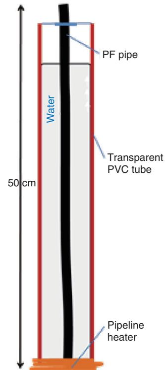
Fig. 4. Lifting pipe simulated with transparent PVC tube.
