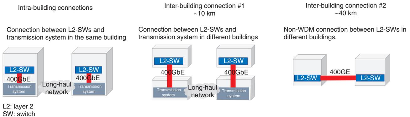
Fig. 3. Application of P2P Ethernet interfaces (telecom networks).
