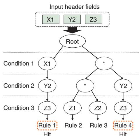
Fig. 4. Network-traffic classification using search tree.
