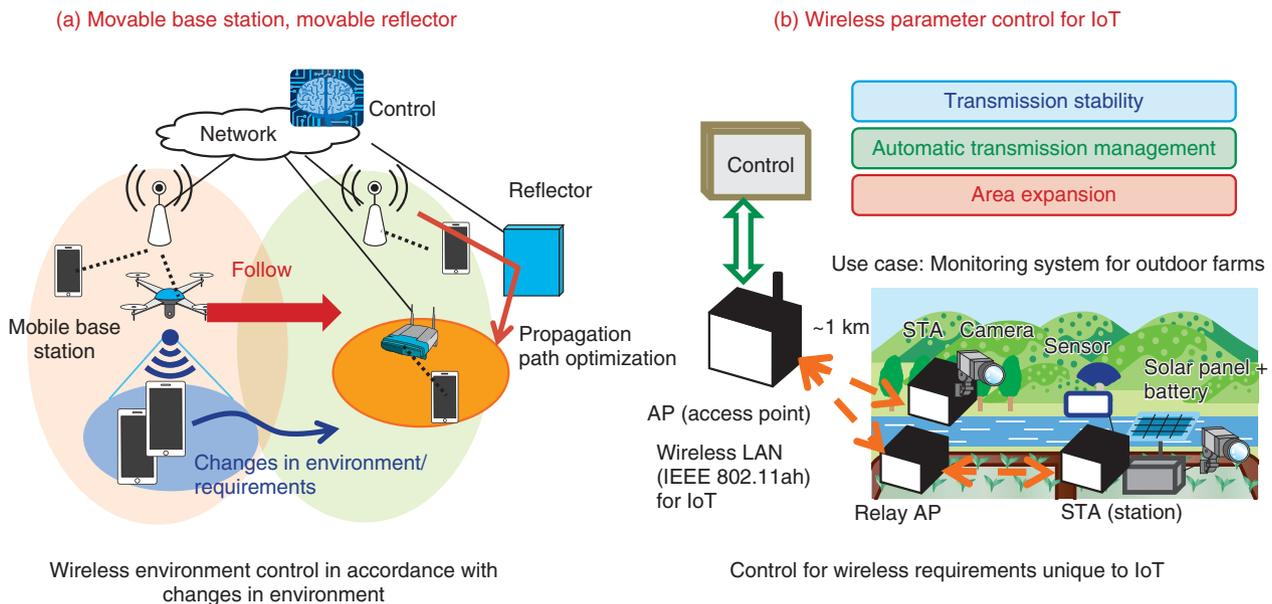
Fig. 5. Wireless-network dynamic design/control technologies.
