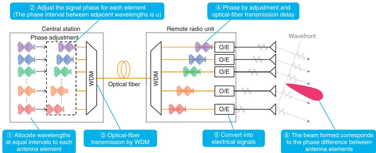
Fig. 1. Remote beamforming scheme with fixed wavelength allocation.
