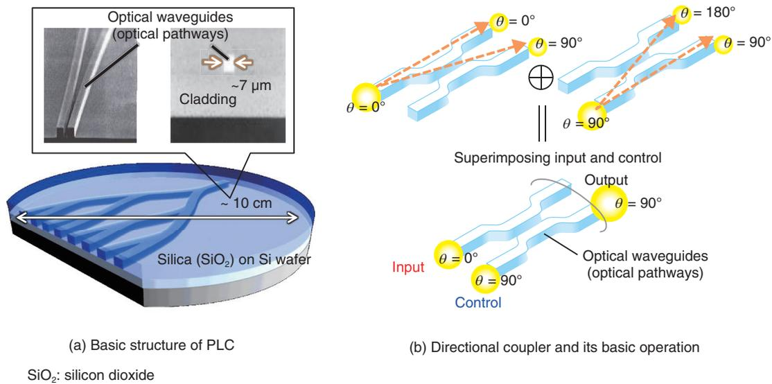
Fig. 1. PLC and basic operation of directional coupler.
