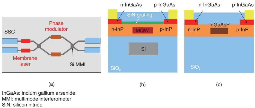
Fig. 2. (a) Schematic diagram of photonic integrated circuit including MZ modulator and membrane laser. (b) Cross-sectional view of membrane laser. (c) Cross-sectional view of phase modulator.
