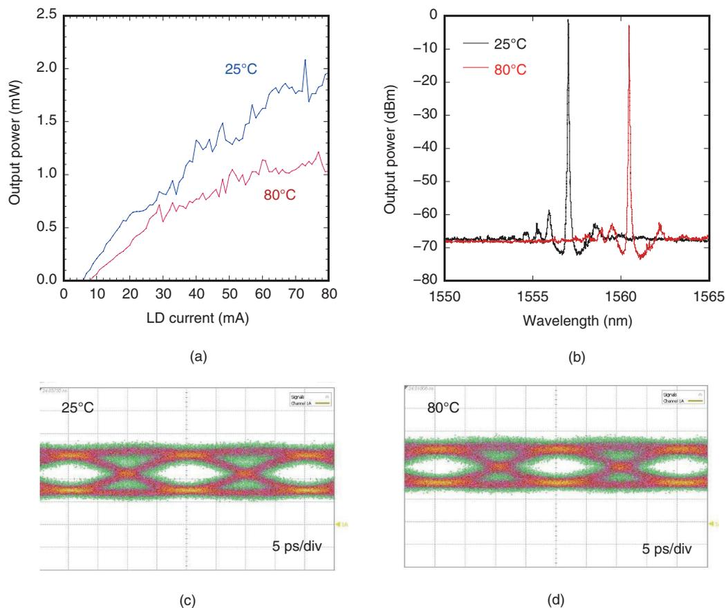
Fig. 4. Characteristics of fabricated device. (a) I-L characteristics at 25 and 80°C. (b) Lasing spectra. (c), (d) Eye diagrams with 50-Gbit/s NRZ signals at 25 and 80°C.
