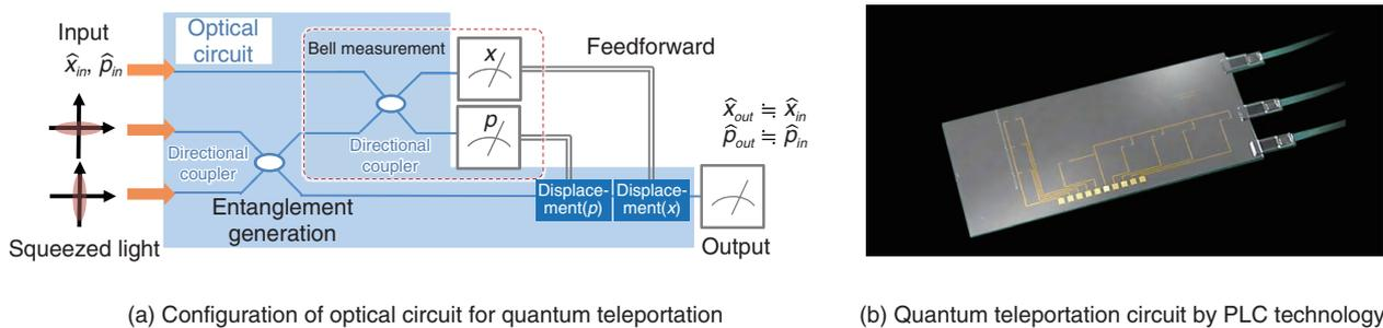
Fig. 4. Optical circuit for continuous-variable-type optical quantum information processing.
