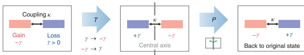
(a) PT symmetry of a system of two coupled cavities.  $\kappa$ : coupling rate.  $\gamma$ : loss rate in a single cavity mode (a negative value represents gain).
