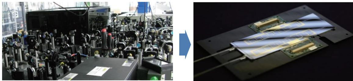
(a) Optical circuit by spatial optics with mirrors and lenses (left), and PLC for universal (right)
