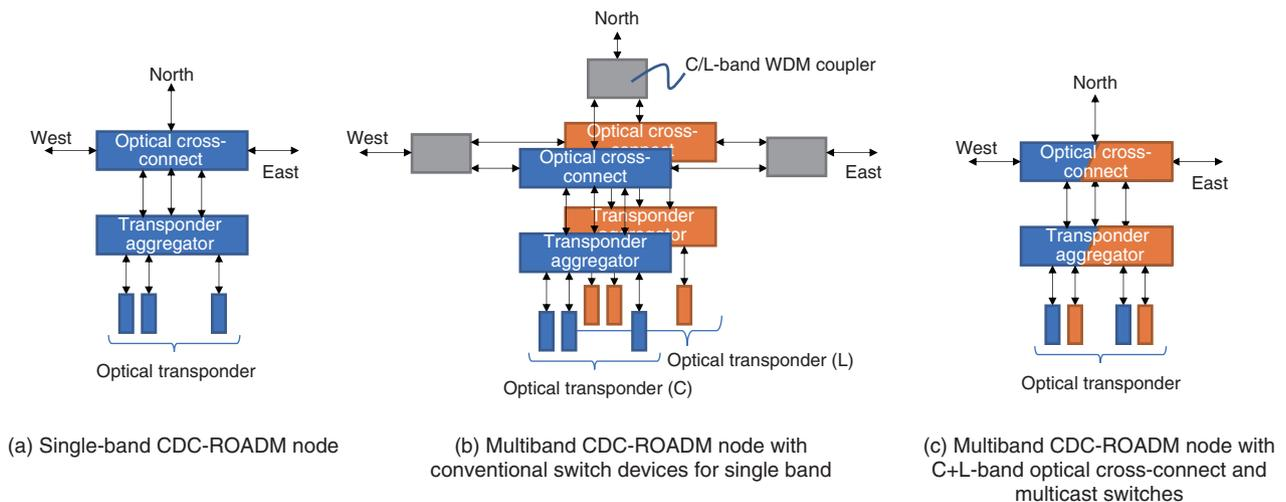
Fig. 3. Configuration of multiband CDC-ROADM node.
