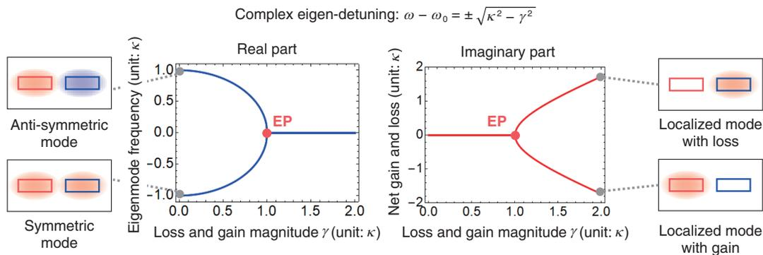
(b) EP transition of the eigenmode frequency and net gain and loss. The red and blue ellipses in the mode schematics represent antiphase fields.  $\omega_0$ : resonance frequency of each cavity mode.
