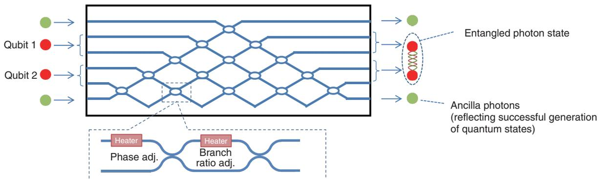
(b) Configuration of generating entangled photon state with optical circuit by PLC
