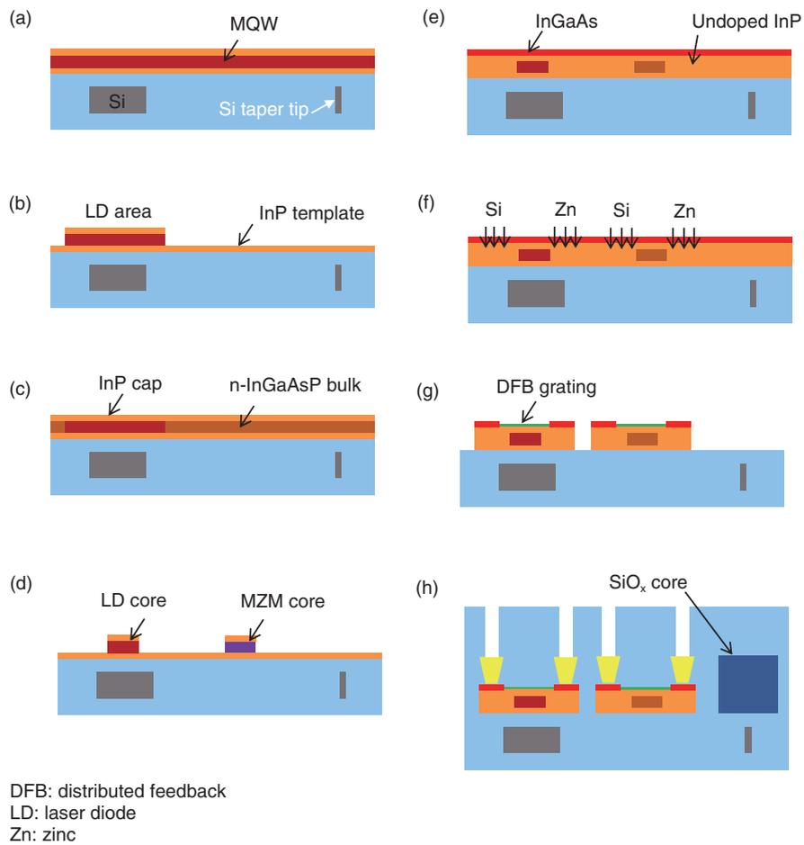
Fig. 3. Fabrication procedure.
