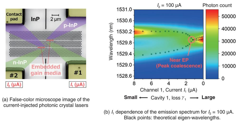
Fig. 2. EP phase transition of current-injected photonic crystal lasers.
