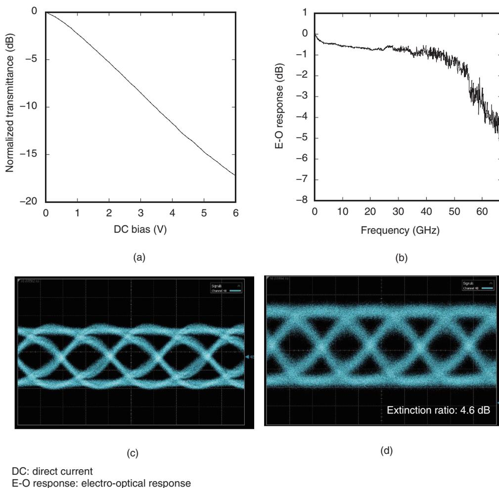
Fig. 5. Characteristics of fabricated EAM. (a) Voltage dependence of transmittance at operating wavelength of 1280 nm. (b) Small signal response at bias current of 2 V. (c) Input electrical and (d) output optical eye diagrams with 100-Gbit/s NRZ signals.
