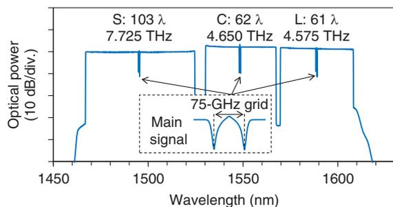
Fig. 3. WDM signal spectra of 16.95-THz bandwidth.
