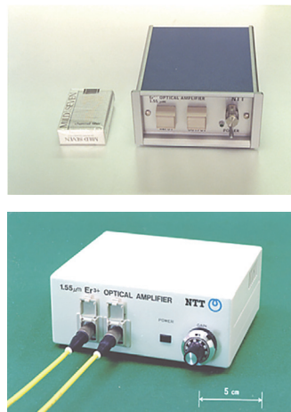
Fig. 1. World's first semiconductor-laser-pumped EDFA.
