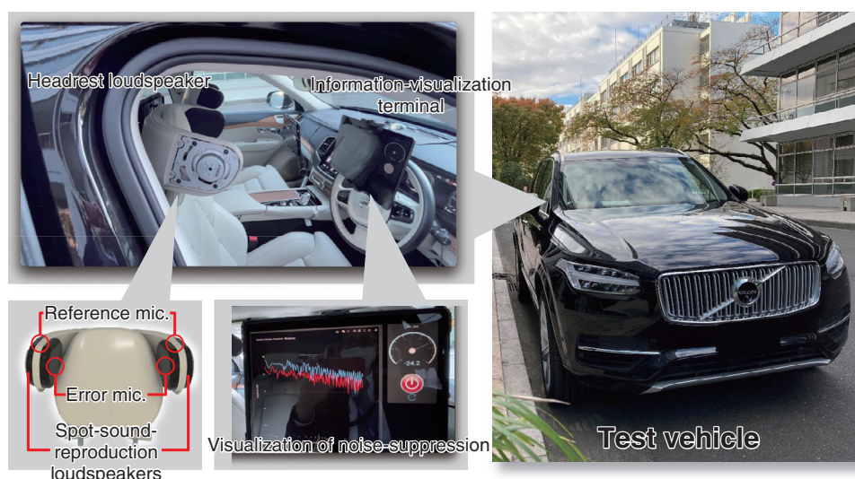
Fig. 5. Example of implementing an ANC system that does not block the ears.
